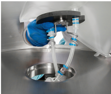
Figure 4. Sparge line support.
