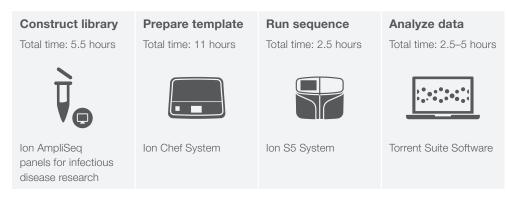
Figure 1. Ion AmpliSeq workflow. Ion AmpliSeq libraries are prepared manually or with the Ion Chef System. Libraries are then placed in the Ion Chef System for emulsion PCR, enrichment, and loading onto Ion S5™ Chips.
