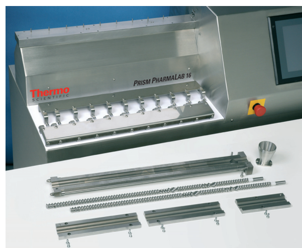
Figure 2: Extruder with all process contact parts removed
