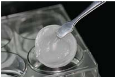
Figure 2—Firm Algimatrix™ sponge from a 6-well plate format can be easily transferred for downstream processing.
