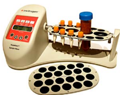
Figure 1. The versatile HulaMixer™ Sample Mixer comes with two tube holder plates to suit all kinds of microtubes and vacutainers (0.5–50 mL).
