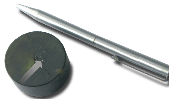
Figure 3: Glass sample with shiny inclusion
