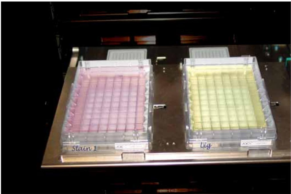
**Figure 3.13** Stain 2 Tray and Fix Tray loaded in drawer 4.
