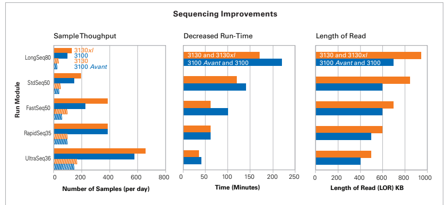
Figure 1. Improved Sequencing Throughput and Length of Read with Decreased Run Times by Upgrading to the 3130 Series Genetic Analyzer
