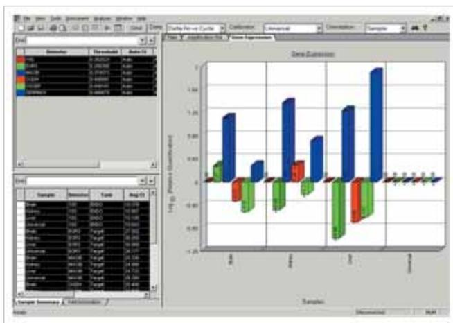
**Figure 5.** Display of  $\log_{10}$  fold change in gene expression for five genes from four samples using the 7500 Fast System in fast mode. Run time: 37 minutes.
