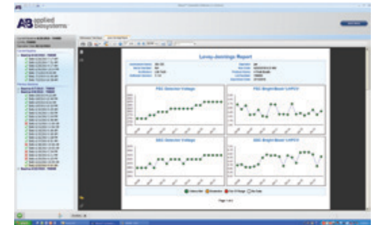
Figure 10. Example of Levey-Jennings plot showing Attune® cytometer performance over time. This report is generated using data from performance tracking beads.
