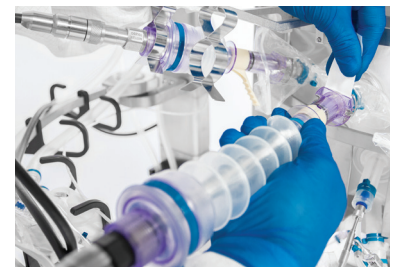
Figure 6. Bioreactor probe assembly.
