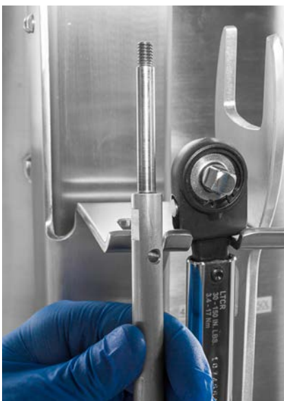
Figure 2.9. Stored tools and multiple-section drive shaft.
