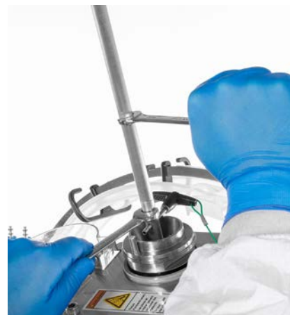
Figure 3.29. Reverse-threading of second segment of multi-segment drive shaft.
