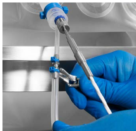
Figure 3.20. Attaching the ground clip to the metal insert on the sample line.
