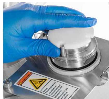
Figure 3.27. Aligning with the keyway.
