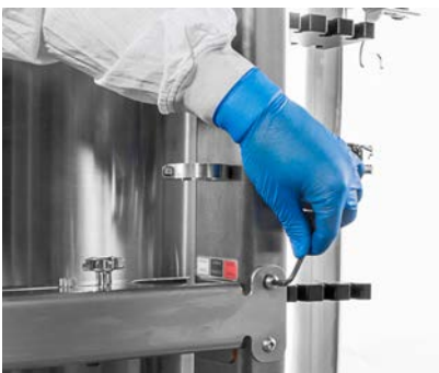
Figure 2.5. Attaching the cable management arm onto the beam.
