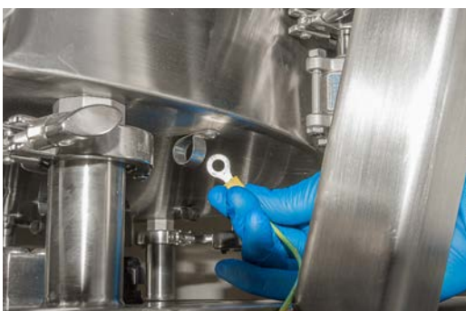
Figure 2.28. The connection of the ground wire from the controller to the bottom of the S.U.M.
