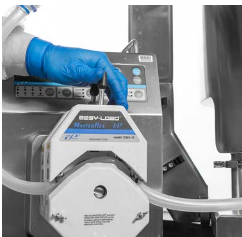
Figure 3.11. Drain line in peristaltic pump.
