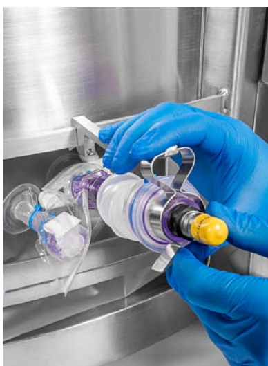
Figure 3.22. Placing collapsed probe assembly into the clip.
