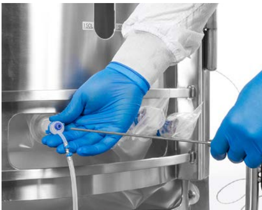
Figure 3.15. Inserting the RTD.
