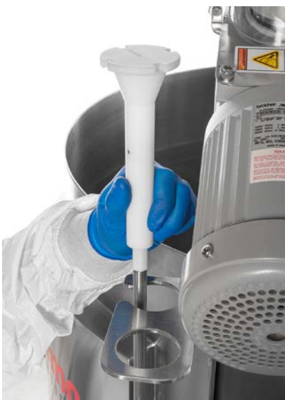
Figure 2.11. Storage of single-section drive shaft.
