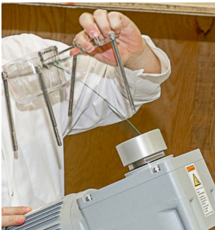
Figure 2.2. Safety cap mounting plate with bolts.
