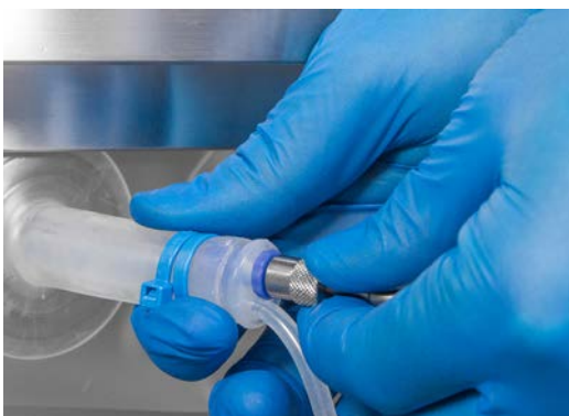
Figure 3.16. Twisting the RTD to secure.
