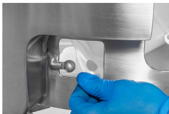
Figure 3.8. Aligning BPC positioning tabs with pins.
