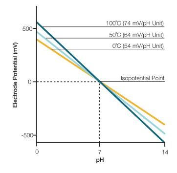
dependent chemical equilibria. The pH electrode should be calibrated with buffers that have known pH values at different temperatures.
