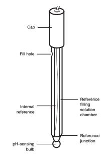
Figure 1 – Typical pH Electrode Components
