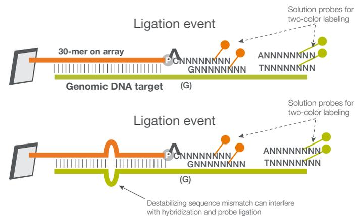
**Figure 1. Schematic illustration of Axiom chemistry in the absence of a secondary polymorphism (above) and in the presence of a secondary polymorphism (below).**
