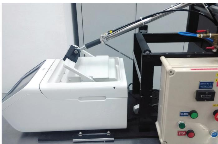
**Figure 1. ProFlex PCR System instrument in “lid actuation robot”.** This testing involves repeated opening and closing of the heated cover to determine the lifespan of the lid mechanism.
