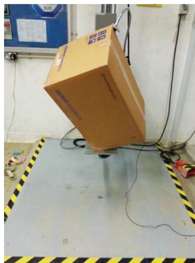
Figure 3. ProFlex PCR System shown in shipping box drop testing.
