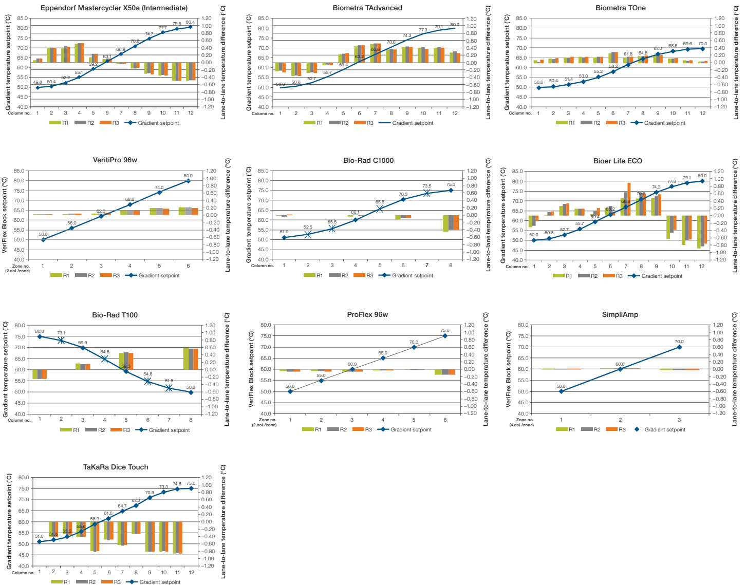
Figure 6. Measured temperature profiles across thermal cycler metal blocks.
