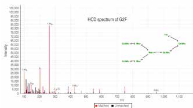
Figure 6. Identification and structural confirmation of released glycan using high resolution HCD MS/MS
