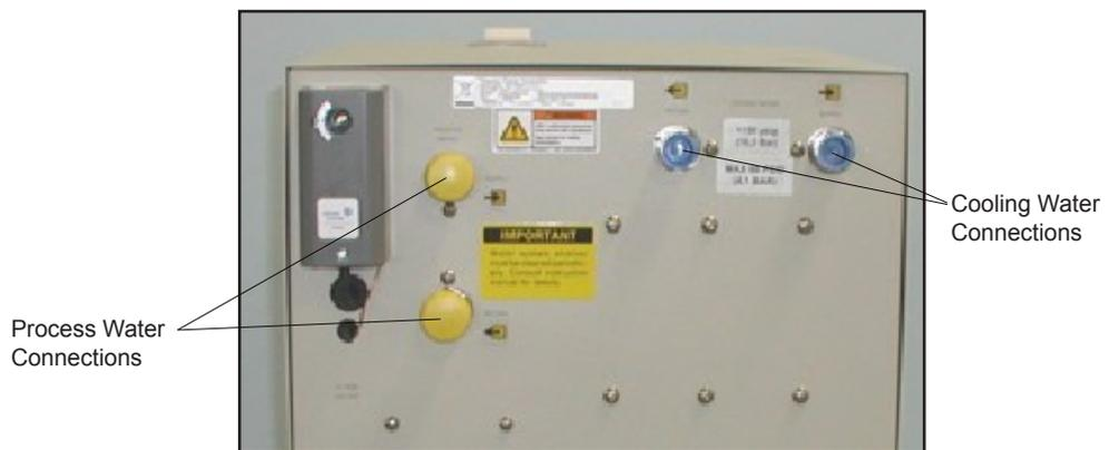
Flexible tubing, if used, should be of heavy wall or reinforced construction. All tubing should be rated to withstand 80 psi at  $+35^{\circ}\text{C}$ . Make sure all tubing connections are securely clamped. Avoid running tubing near radiators, hot water pipes, etc. If substantial lengths of tubing are necessary, insulation may be required to prevent loss of cooling capacity.
