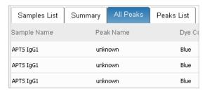
**4.** Examine the **Peaks list** tab for a list of peaks that meet the **Peak Amplitude Threshold** in the analysis method and the **RMU** value for each peak.
