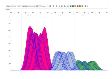
7. Click to display individual traces, then scroll through each individual trace to confirm that the peaks are correctly selected.
