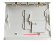
**6.** Place the stack including the tray on the instrument blotting surface. Align the copper tab with the  $\bigoplus$  symbol.
