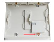
**6.** Place the stack including the tray on the instrument blotting surface. Align the copper tab with the + symbol. [2]
