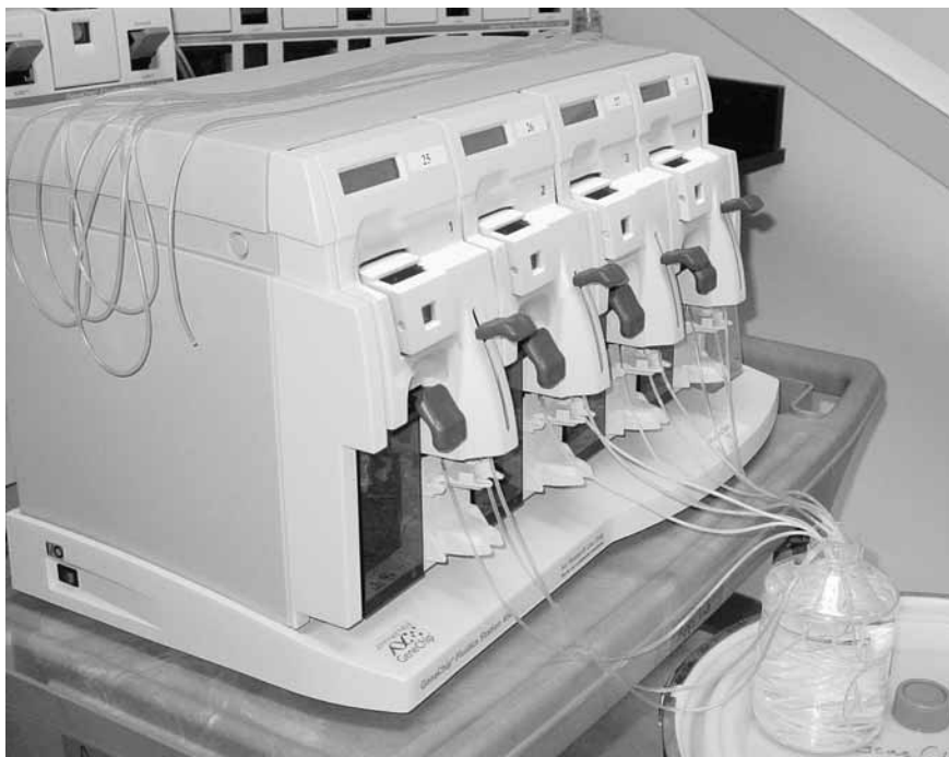
Figure 6.3 The tubes extending from the modules to the bleach bottle. Note that the probe array cartridges must be removed before the protocol can begin.
