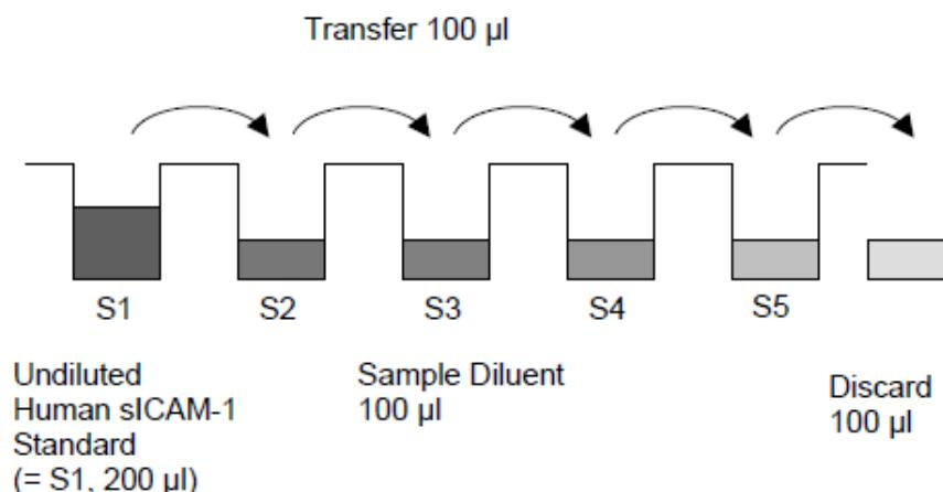
In case of an **external standard dilution** (see 9.4.1), pipette 100 µl of these standard dilutions (S1 – S5) in the standard wells according to Table 1.
