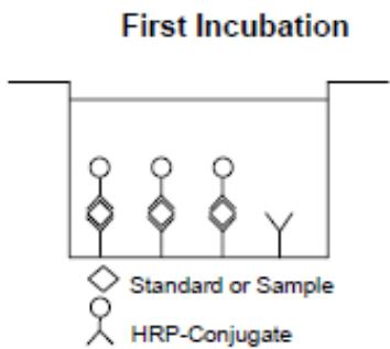
Following incubation unbound HRP-conjugated anti-human sICAM-1 is removed during a wash step, and substrate solution reactive with HRP is added to the wells.
