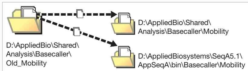
Figure 1-3 Where to copy 310 DyeSet/Primer files
