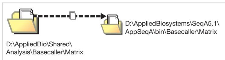
Figure 1-4 Where to copy 377 matrix files
