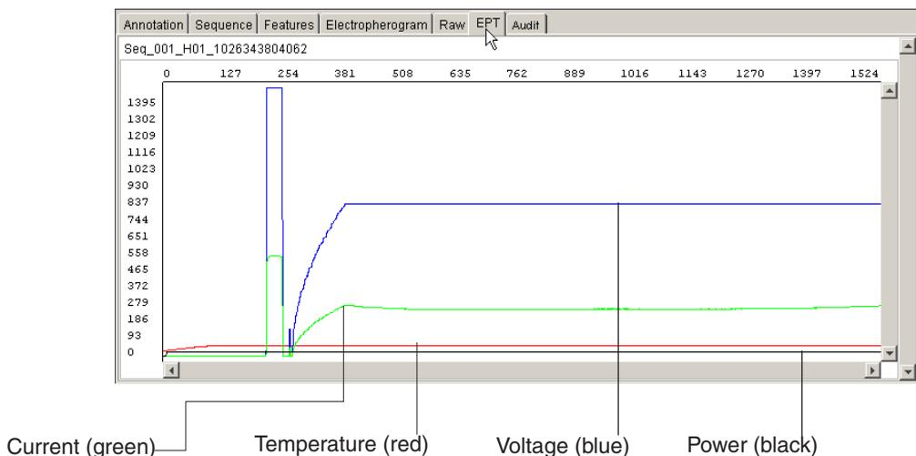
Figure 3-11 Single sample in the EPT view
