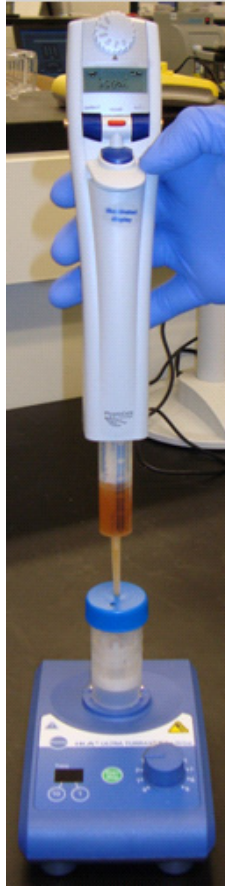
Figure 13 Correct placement of Combitip Plus into sample port in SOLiD™ ePCR Tube cap.
