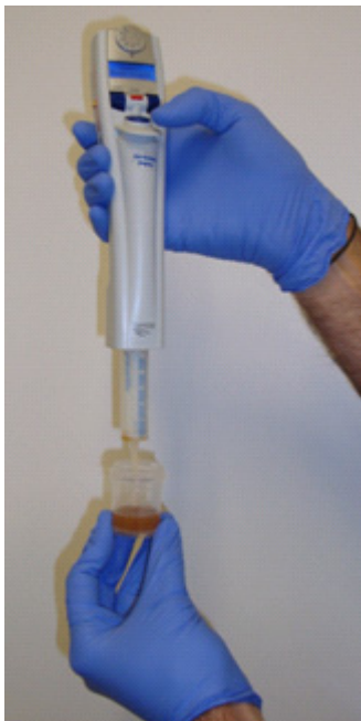
Figure 24 Filling the 10-mL Combipip Plus tip with the aqueous phase and bead mixture using the Xstream pipettor.
