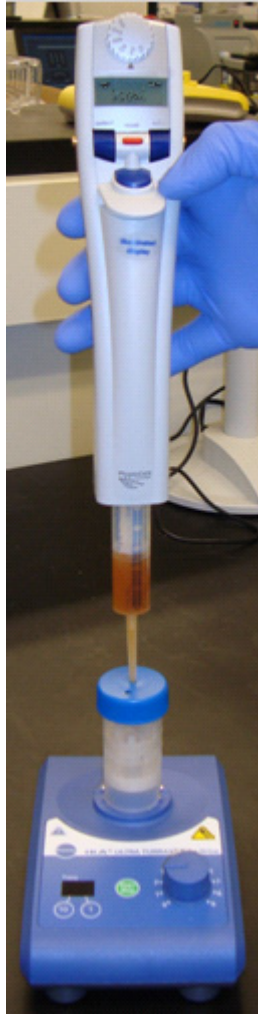
Figure 25 Correct placement of Combitip Plus into sample port in SOLiD™ ePCR Tube cap.
