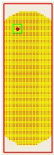
Figure 71 Use the mouse to drag the green-box cursor and to move the flowcell stage the same way.
