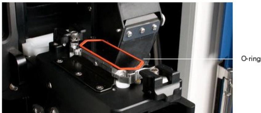
Figure 21 O-ring installed on flowcell.
