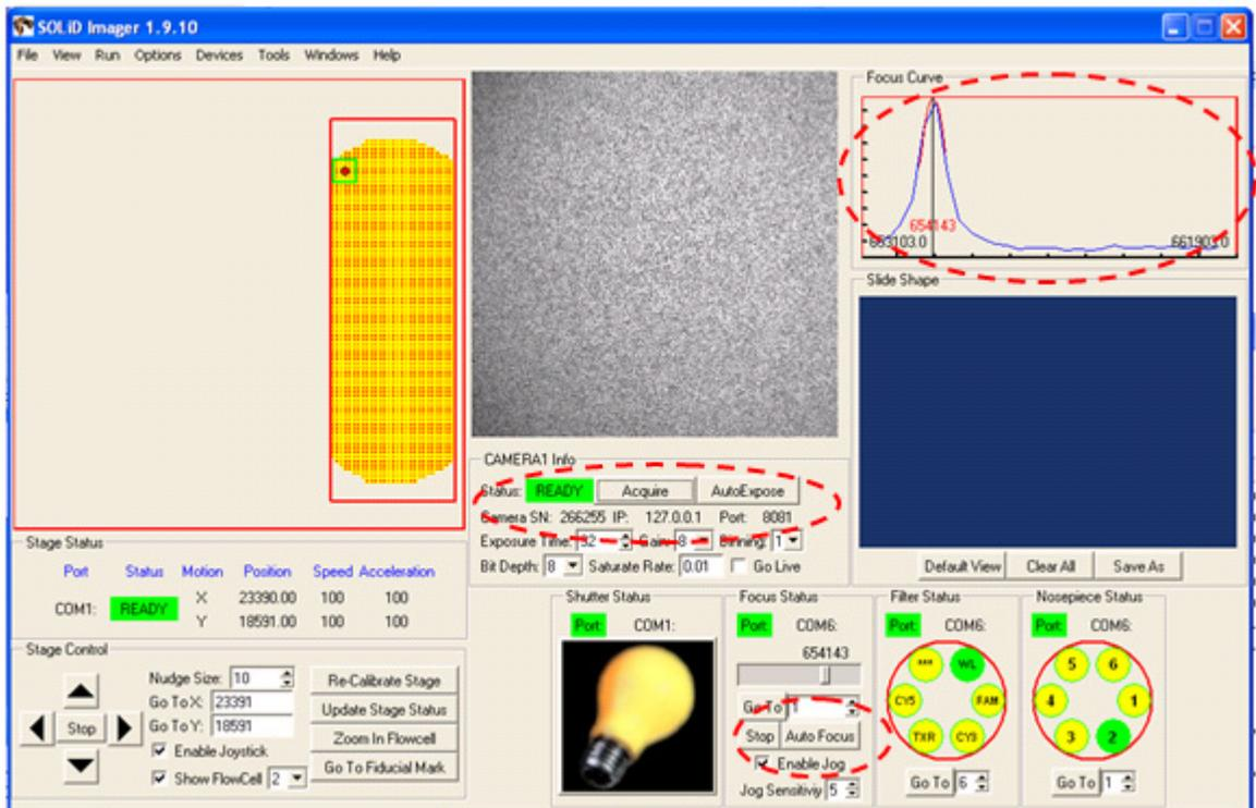
Figure 73 Click **AutoFocus** and **AutoExpose** so that the focus peak falls in the focus range.
