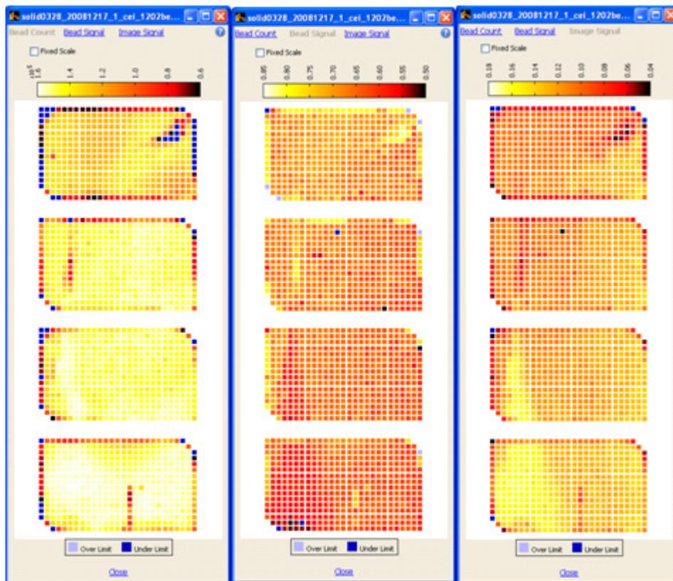
Figure 63 Bead Count (left), Bead Signal (center), and Image Signal (right) heat maps.
