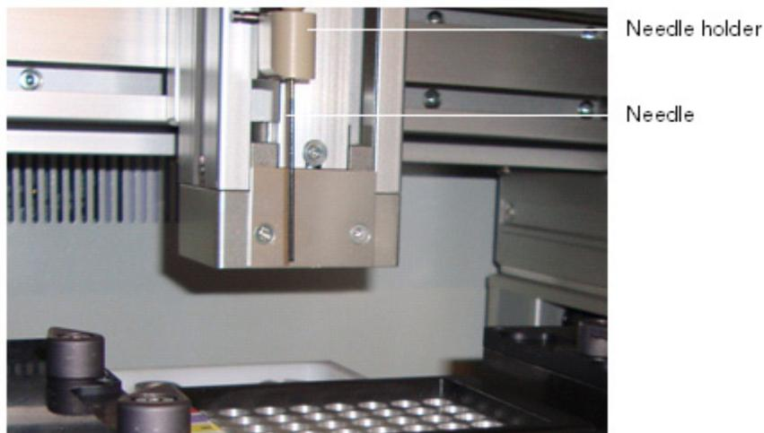
Figure 24 Needle and needle holder.
