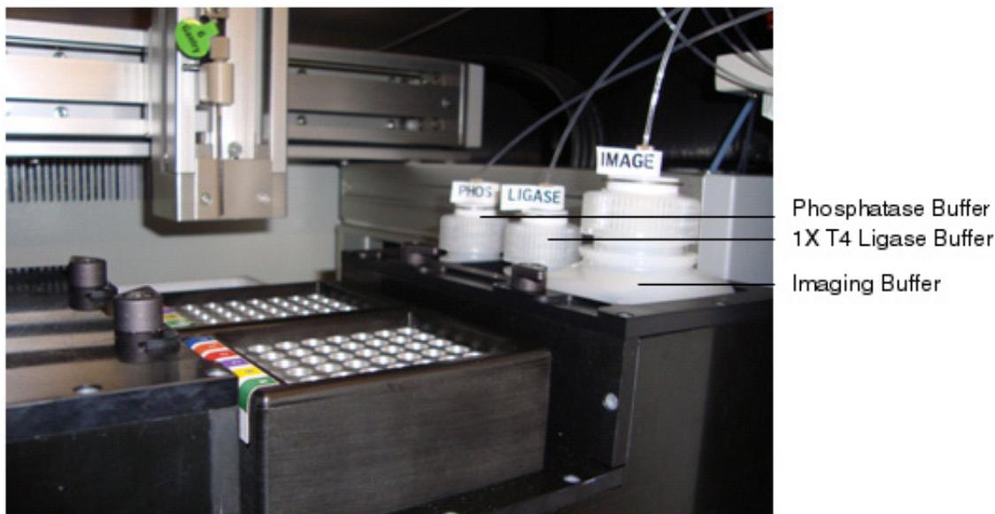
Figure 16 Positions of buffer bottles in the chiller block.
