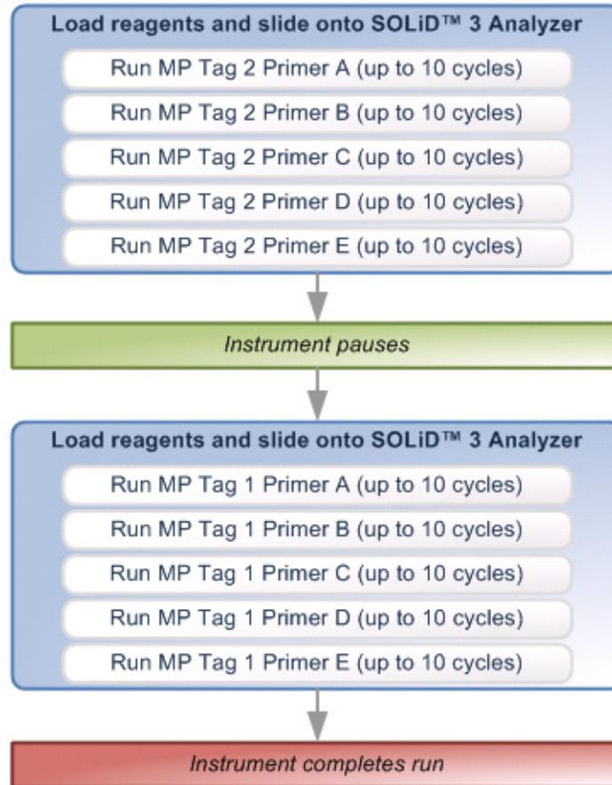
Figure 5 Typical workflow of a mate-paired sequencing run.
