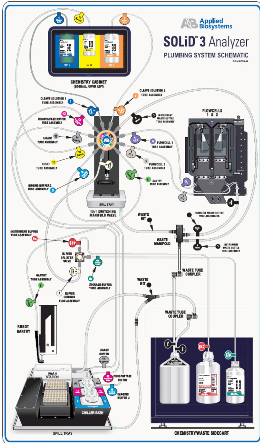
Appendix E SOLiD™ 3 Analyzer Plumbing System Schematic
