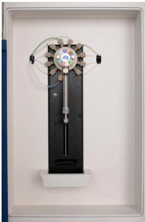
Figure 18 Syringe on the SOLiD™ 3 Analyzer.
