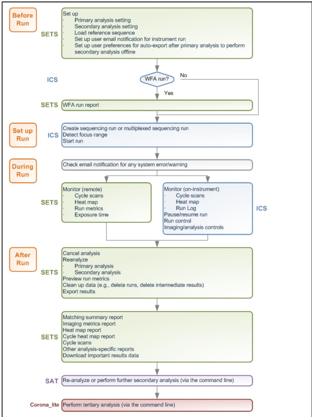
Figure 8 Relationship between software tools in SOLiD™ sequencing run workflow.
