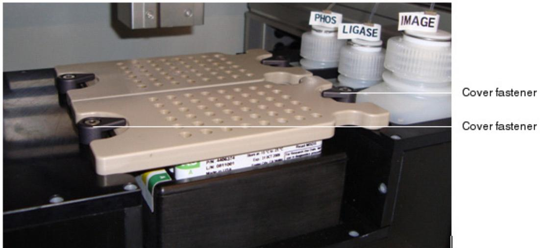
Figure 32 Securely fastened reagent strip covers.
