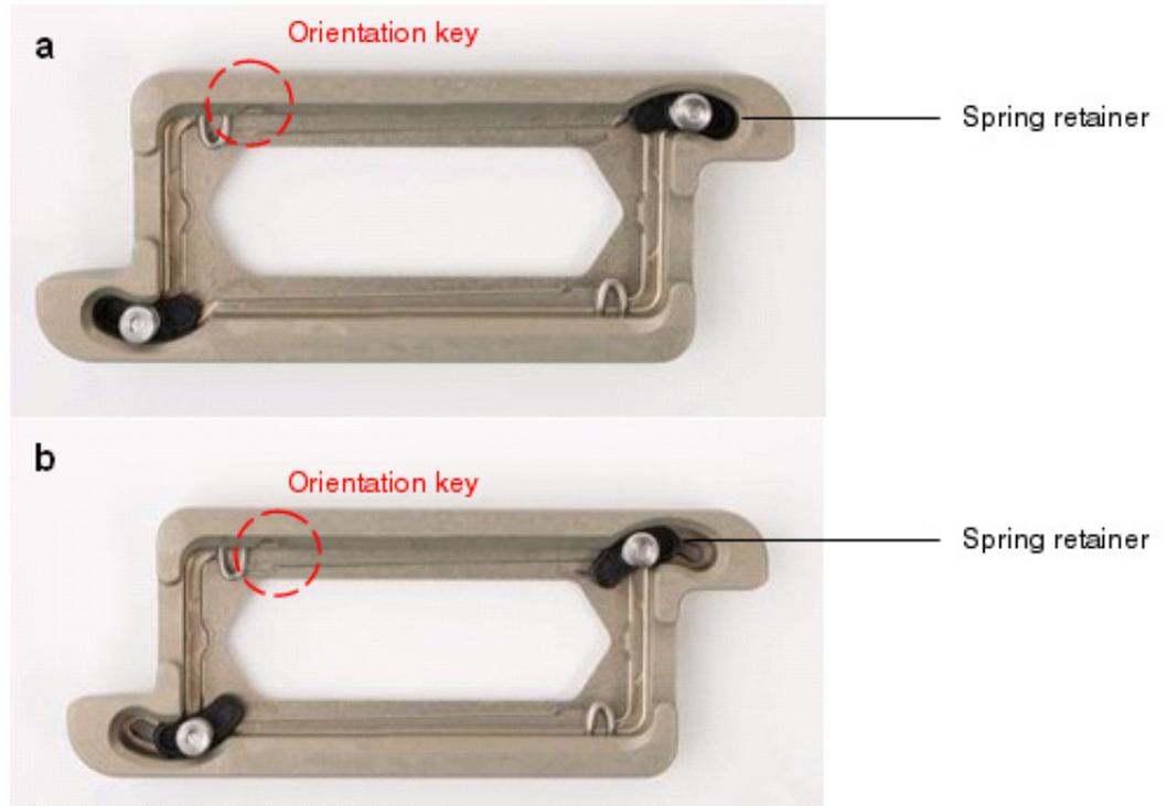
Figure 11 Slide carrier (a) with spring knobs pushed out and (b) with spring knobs pushed in.
