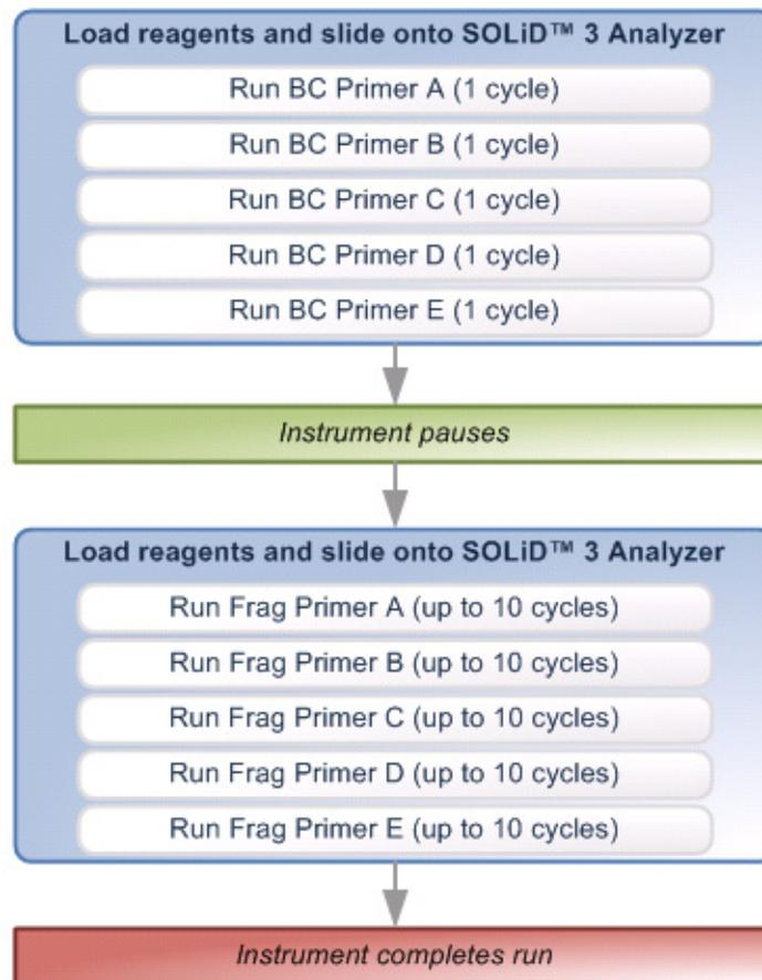
Figure 7 Typical workflow of multiplex fragment sequencing run.
