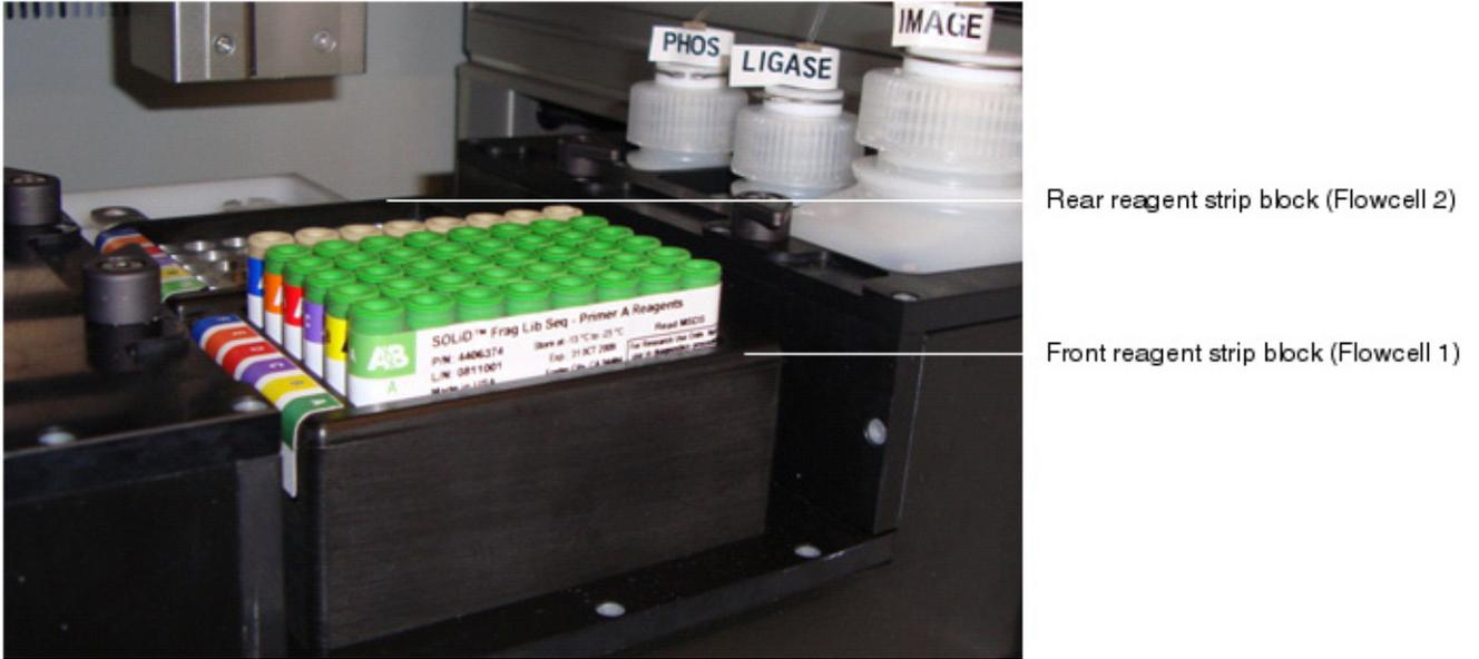
Figure 31 Position of the sequencing reagent blocks for flowcells 1 and 2.
