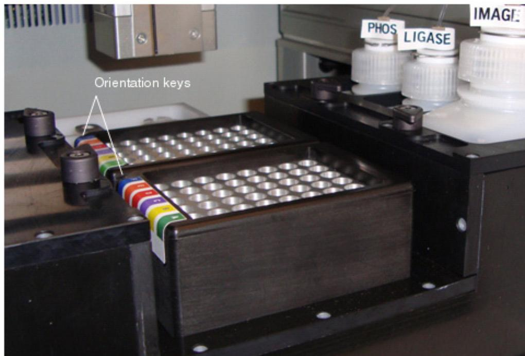
**Figure 30** The Reagent Strip Block.
