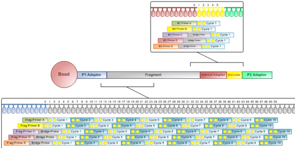
Figure 6 SOLiD™ 3 System interrogation of nucleotide positions for a 50-bp fragment and 5-bp barcode sequencing run.
