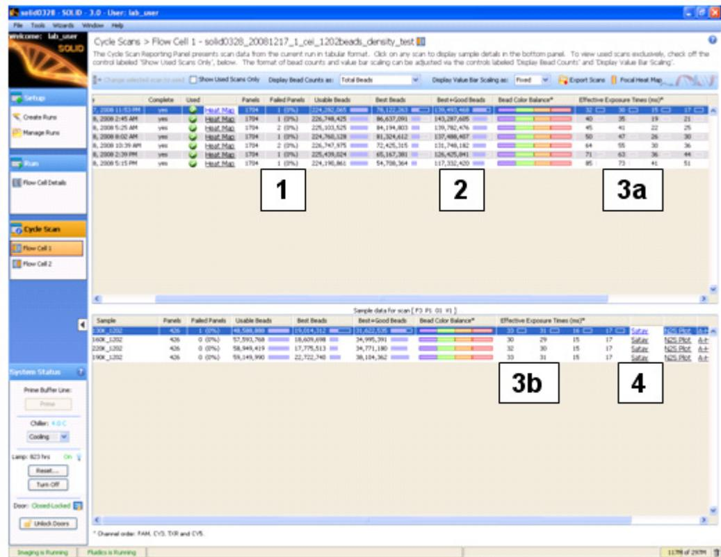
Figure 64 Parameters available in the Cycle Scans window to assess the progress of the sequencing run.
