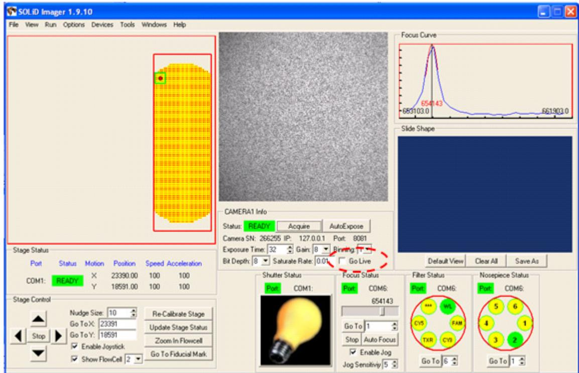
Figure 75 Check **Go Live** to manually find the focal range.
