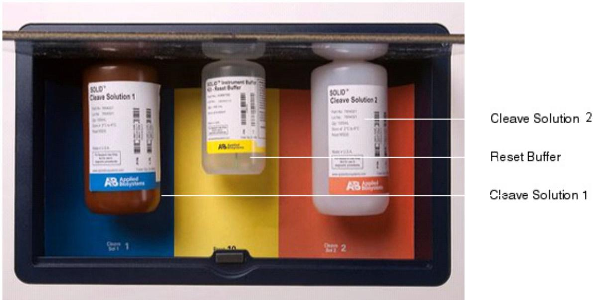
**Figure 15** Positions of reagent bottles on the side of the instrument.
