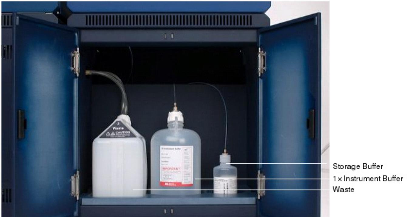
**Figure 14** Positions of buffers and waste in the cabinet.
