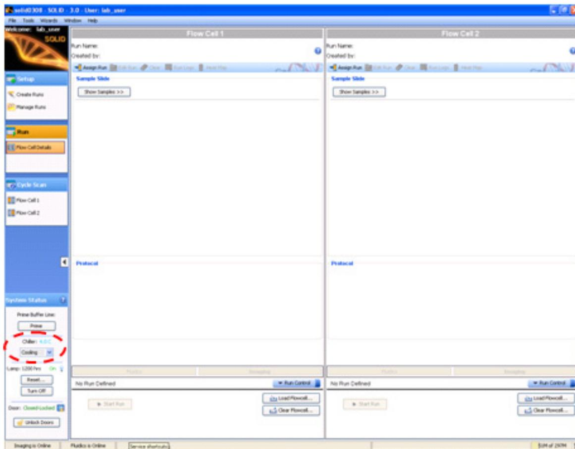
Figure 13 Select **Cooling** to cool the flowcell.
