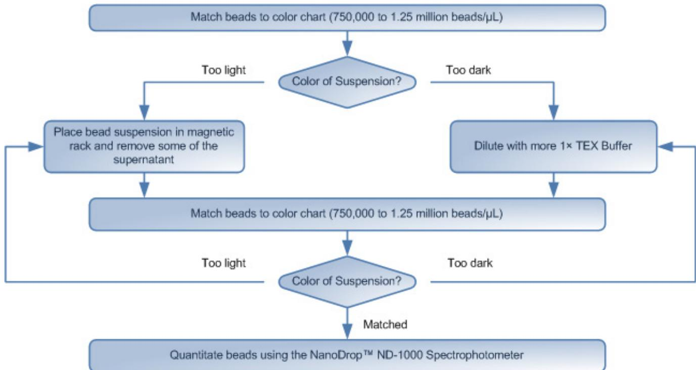
Figure 10 SOLiD™ Bead Concentration Chart workflow.
