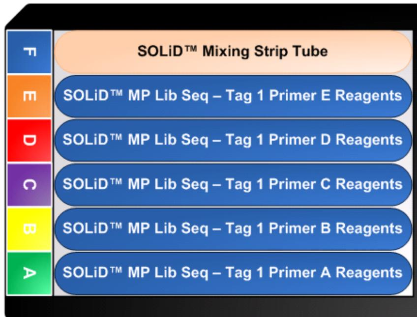
Figure 27 Reagent strip block layout to sequence mate-paired tag 1 (50 bp).
