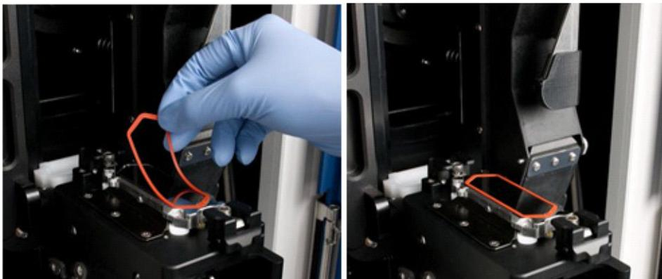
Figure 67 Install the SOLiD™ O-Ring on a flowcell.
