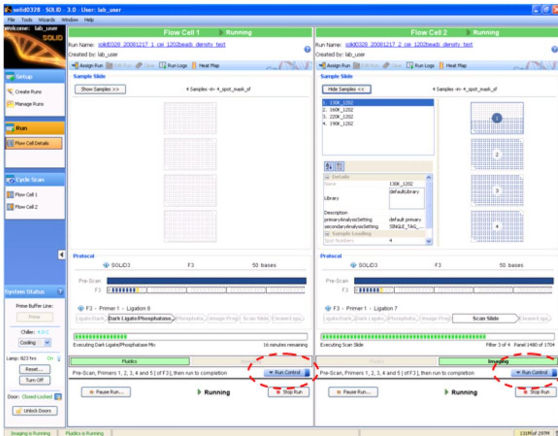
**Figure 60** Click **Run Control** to display the Run Control menu for that flowcell.
