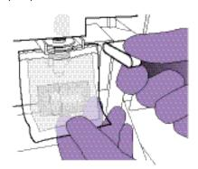
**Note:** The RFID label must face the instrument (away from you) to ensure that the RFID information is read accurately by the instrument.
