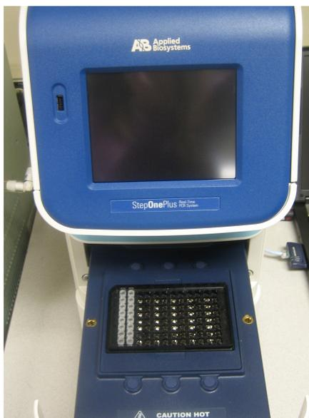
1. Place the MicroAmp® 96-Well Tray for Veriflex™ Blocks (Cat. no. 4379983) on the sample block of the StepOnePlus® System.
