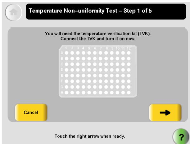
4. Follow the prompts in the touchscreen, making sure the multiprobe module is aligned in the well locations shown on [page 19](#), and as indicated below:
