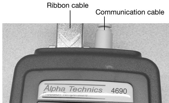
3. Connect the other end of the communication cable (9-pin) to the communication port of the instrument.
