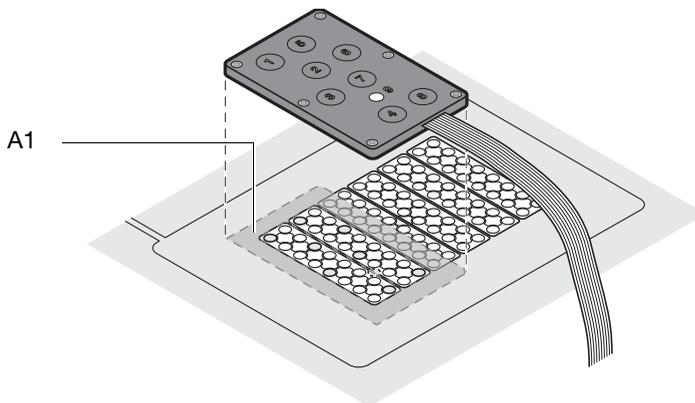
3. Make sure that the ribbon cable leads straight out from the module, lies flat, and is under the thermal cycler cutout.
