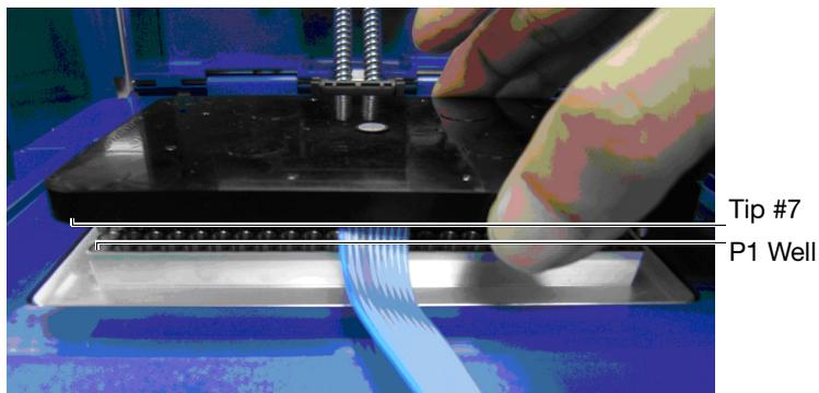
4. Ensure that the ribbon cable leads straight out, lies flat, and is under the thermal cycler cutout.
