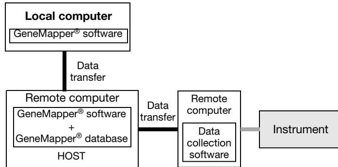
Figure 3-3 Example of stand-alone client configuration
