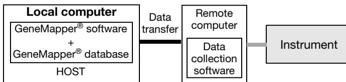
Figure 3-2 Example of a stand-alone configuration
