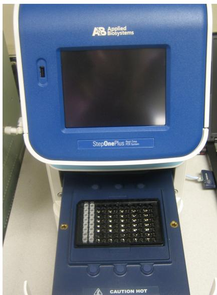
1. Place the MicroAmp® 96-Well Tray for VeriFlex™ Blocks on the sample block of the StepOnePlus™ System.
