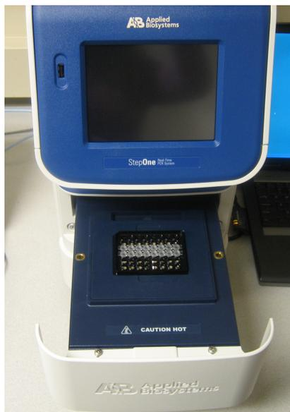
1. Place the MicroAmp® Fast 48-Well Tray on the sample block of the StepOne™ System.
