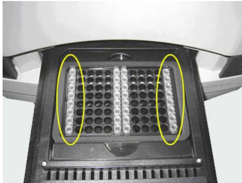
2. Carefully insert two or more 8-tube strips containing samples, starting from the center of the plate holder and moving out. This layout minimizes bending or misaligning the tube strips.
