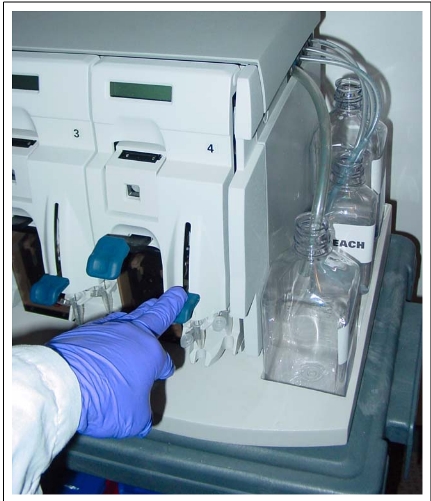
Figure 6.4 Press down on the needle levers to start the bleach protocol.
