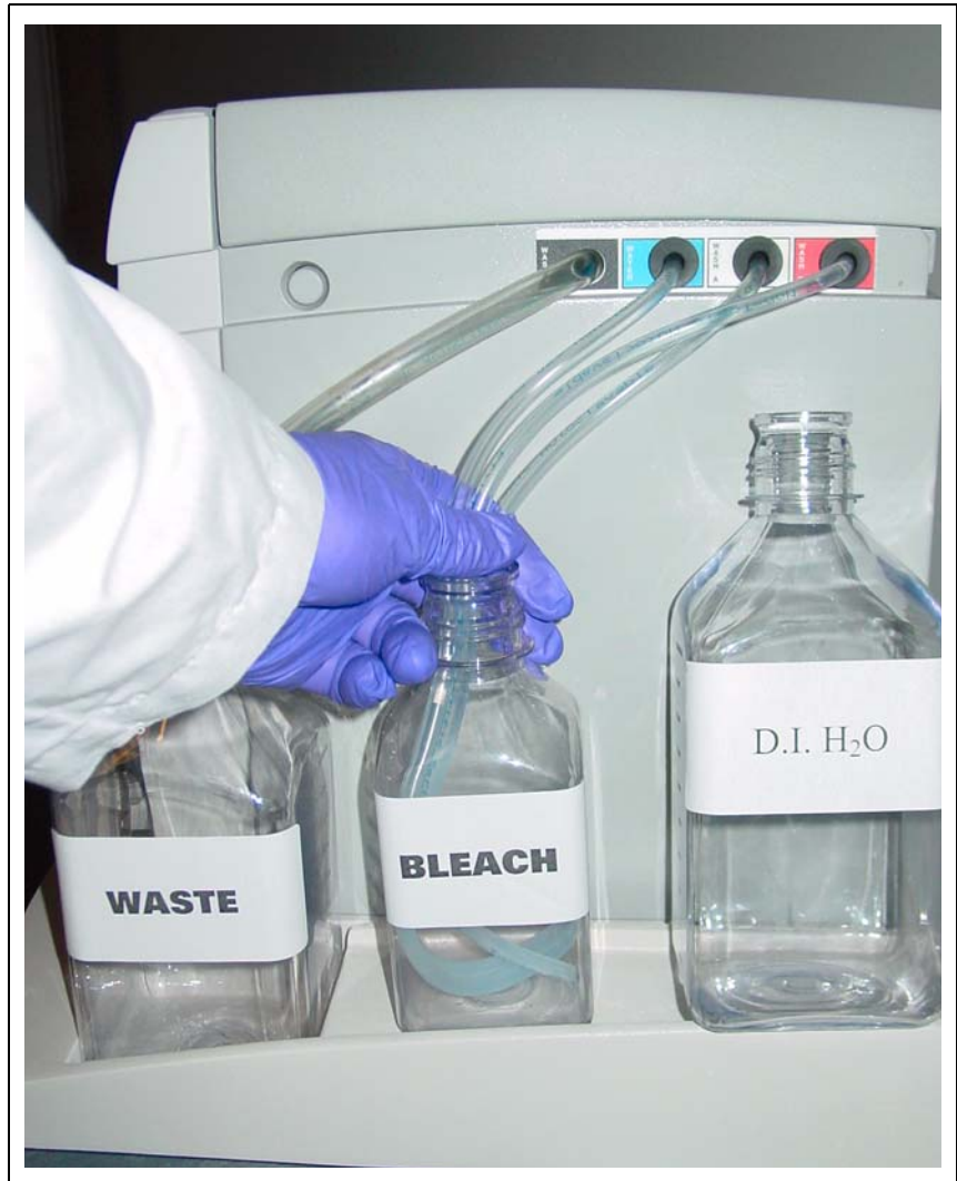
Figure 6.2 The bleach cycle. Immerse the tubes into the 0.525% sodium hypochlorite solution. The waste line remains in the waste bottle.
