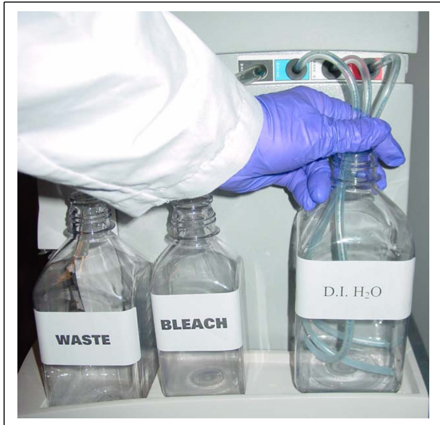
Figure 6.5 Immerse the three wash and water lines in the DI water bottle.
