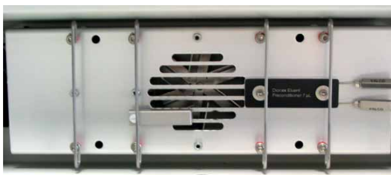
Fig. 9: Eluent preconditioner installed the column chamber (example)
