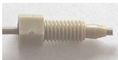
Fig. 1: Capillary with fitting nut and ferrule for connection to the biocompatible valve
