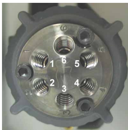
Fig. 23: Connections on a 2-position, 6-port column switching valve
