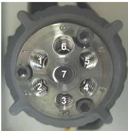
Fig. 25: Connections on a 6-position, 7-port column switching valve
