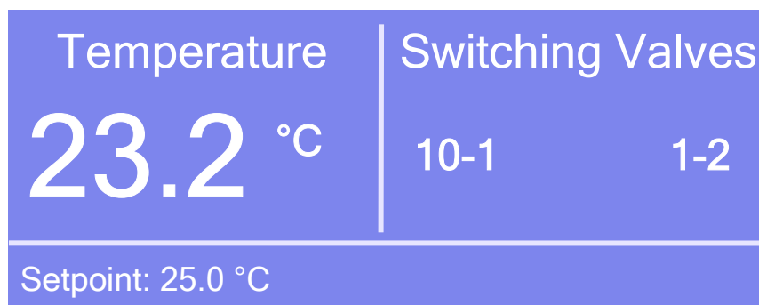
Fig. 31: Status screen (here for a TCC-3200 with two 2-position, 10-port switching valves)
