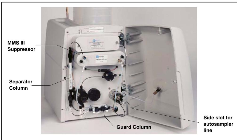
Figure 2-17. ICS-90 with Columns and Suppressor Installed
