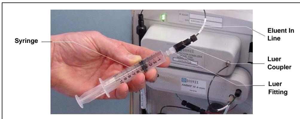
Figure 2-19. Assembled Syringe and Luer Adapter
