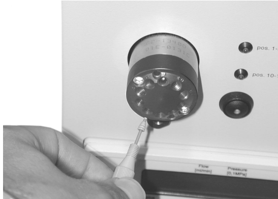
FIGURE G-3 Installing the Pre-assembled Fitting
