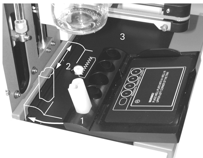
FIGURE 2-5. Installing the Plate Holder
