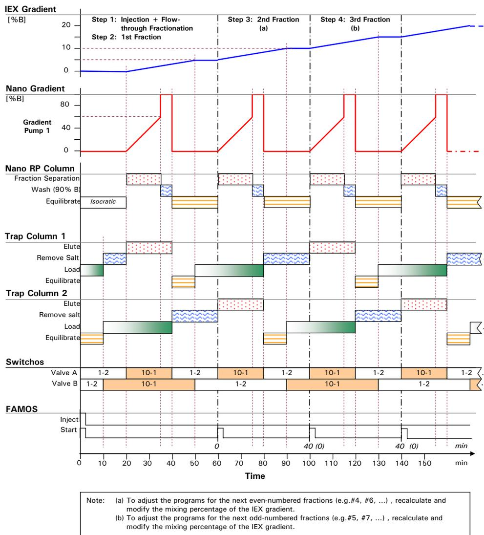
FIGURE 3-3 The First 4 Steps of the Comprehensive 2-D Application
