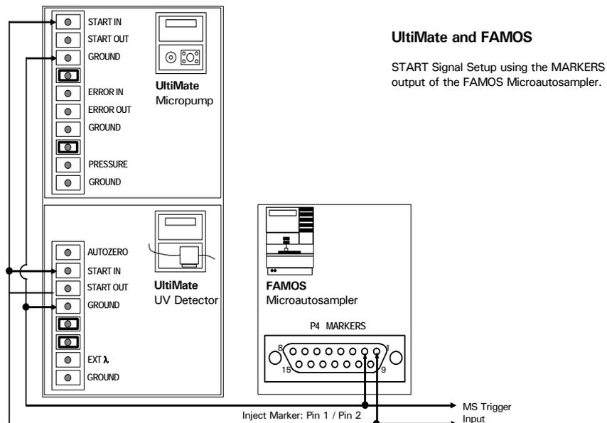
FIGURE 2-3 START Signal Setup – UltiMate and FAMOS
