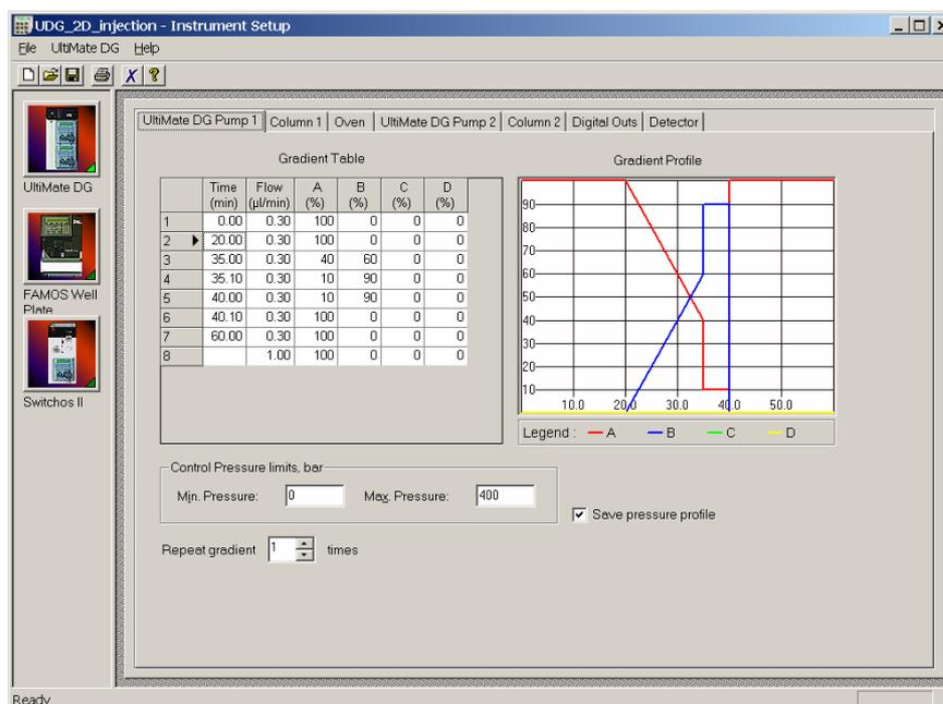
FIGURE 3-4 Gradient Program for the Gradient Pump 1
