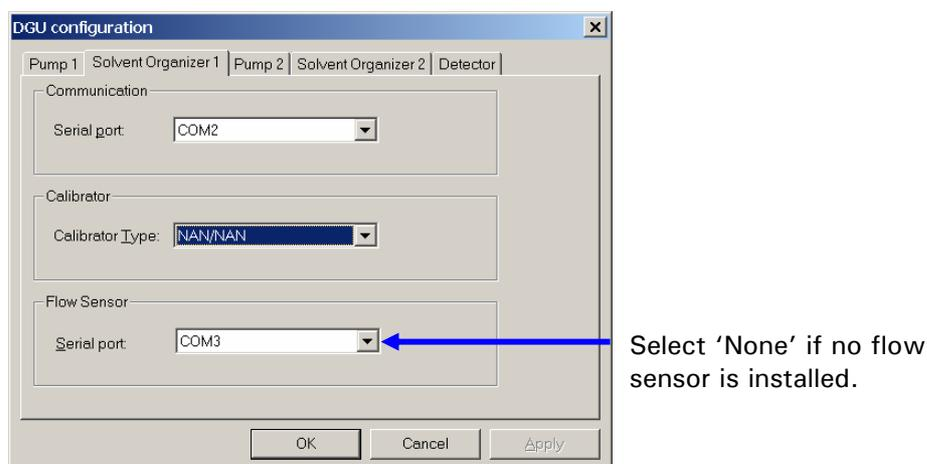
FIGURE 2-20 The UltiMate Solvent Organizer Configuration Window
