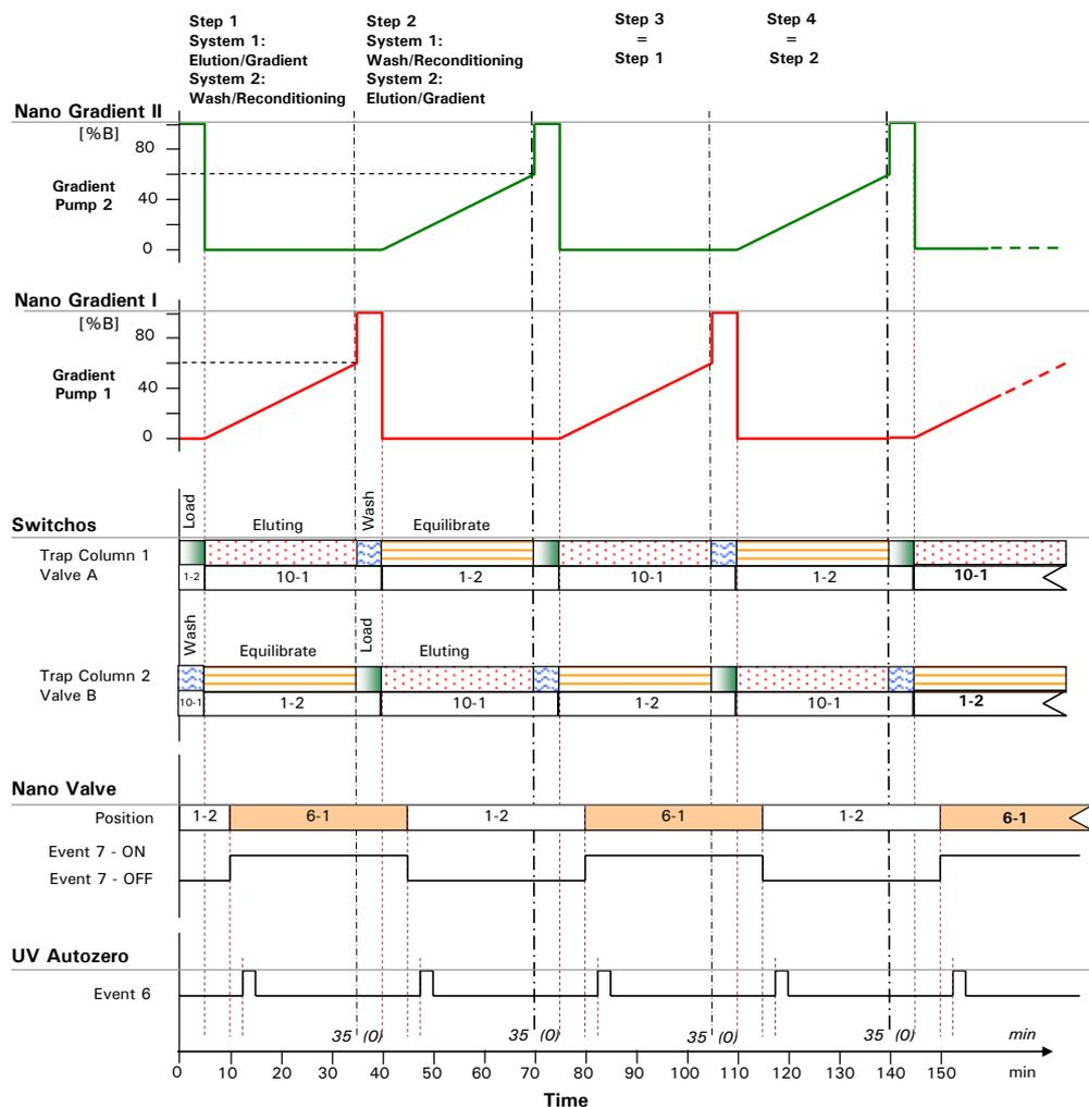
FIGURE 3-14 The First 4 Steps of the Parallel Nano-LC Application
