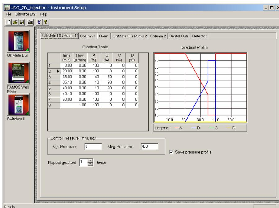
FIGURE 2-32 The Gradient Pump 1 Setup Window
