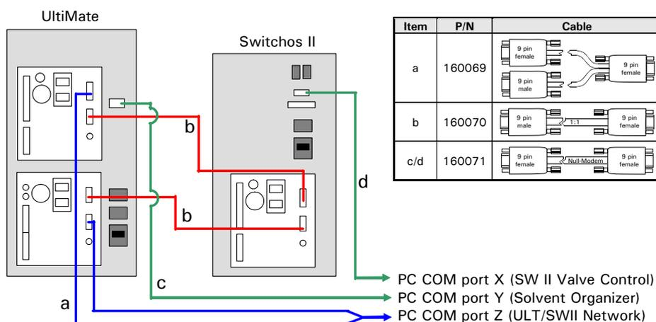
FIGURE 2-1 PC Connections of the UltiMate System (without Flow Sensor) and Switchos
