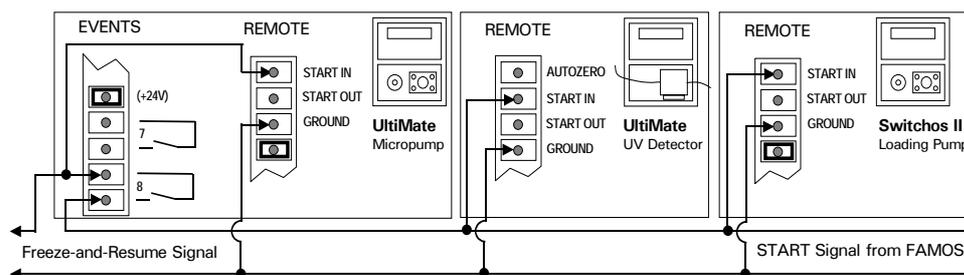
FIGURE 2-6 START Input Setup – Installation including the Peak Parking Kit
