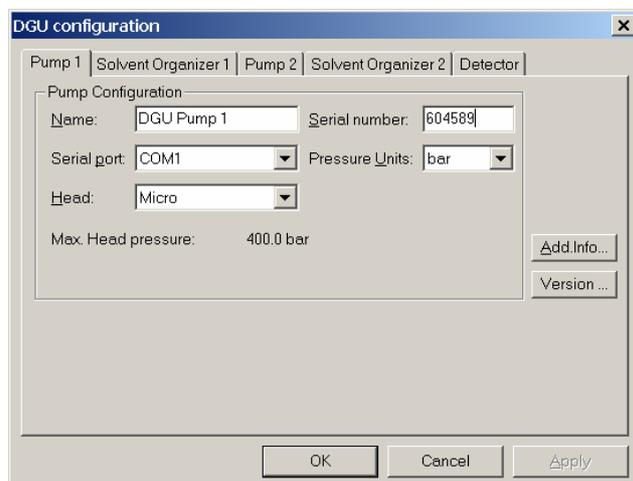
FIGURE 2-18 The UltiMate Pump1 Configuration Window
