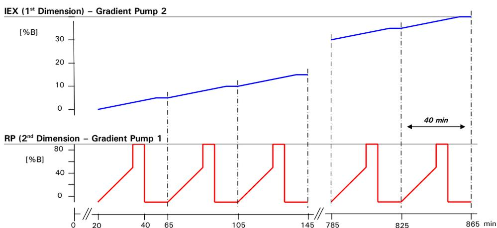
FIGURE 3-2 Gradients used for the Comprehensive 2-D Setup
