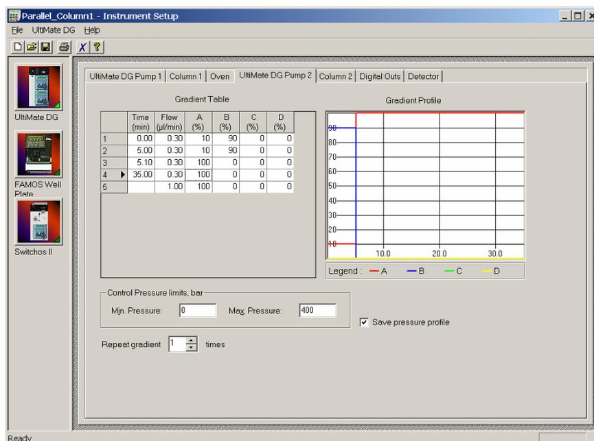
FIGURE 3-16 Gradient Program for the Gradient Pump 2 - Wash and Reconditioning
