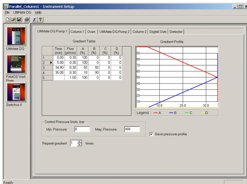
FIGURE 3-15 Gradient Program for the Gradient Pump 1 – Gradient Elution
