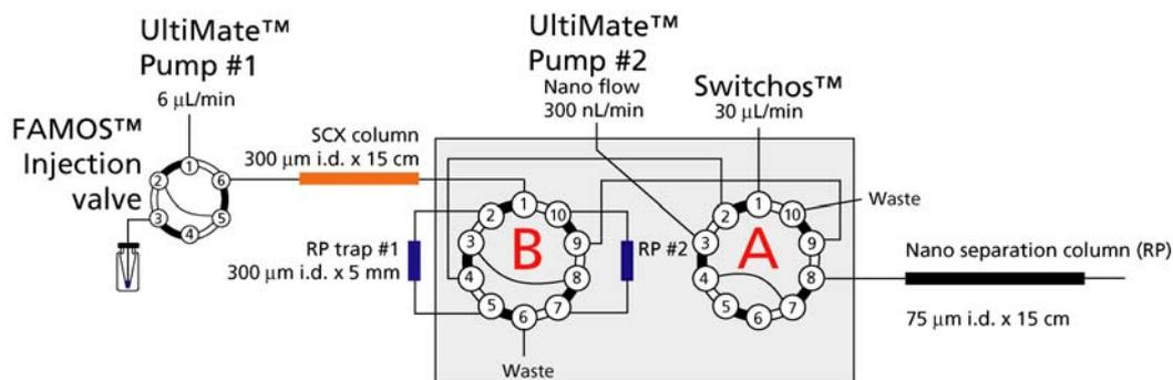
FIGURE 3-1 Fluidic Setup for the Comprehensive 2-D LC Setup
