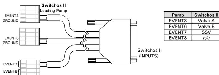
FIGURE 2-7 Switchos II Control Cable
