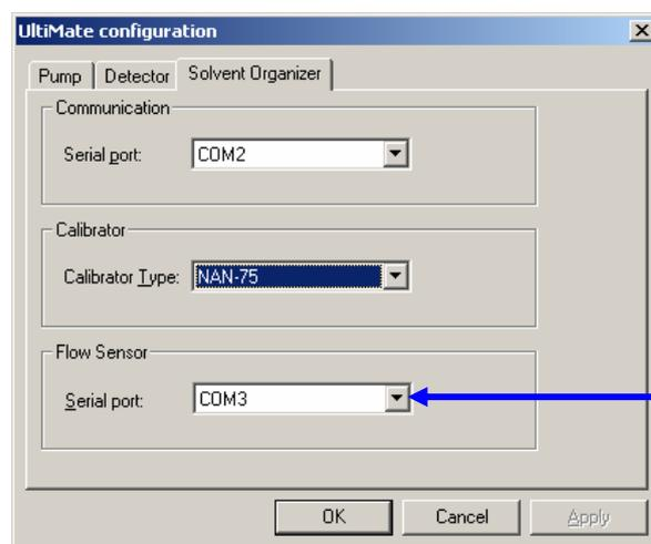
Select 'None' if no flow sensor is installed.
