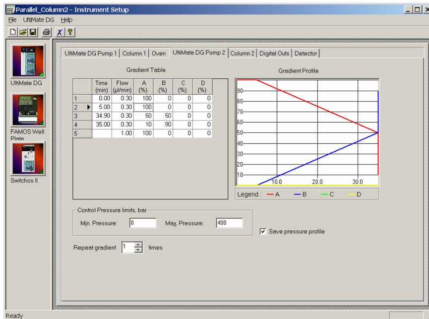
FIGURE 3-23 Gradient Program for the Gradient Pump 2 – Gradient Elution
