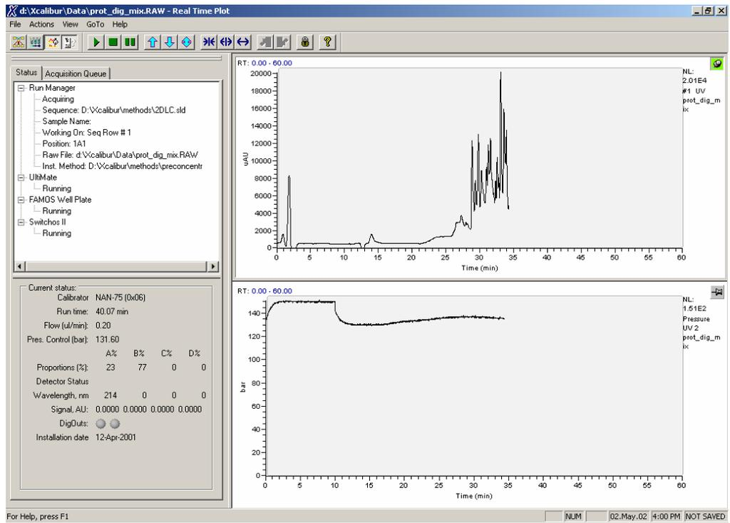
FIGURE 2-49 Presenting the UV Data and the Column Pressure
