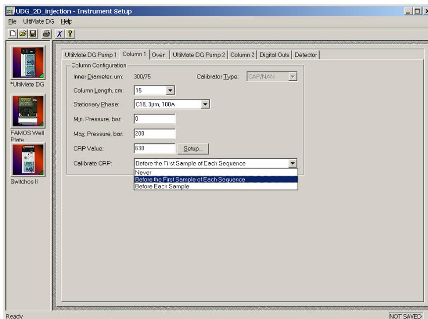
FIGURE 3-6 The Column 1 (Nano Column) Parameters Setup Window
