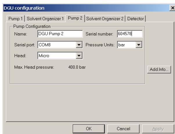
FIGURE 2-19 The UltiMate Pump 2 Configuration Window
