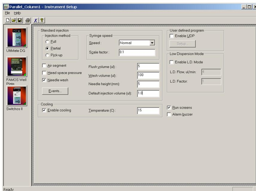
FIGURE 3-21 The FAMOS Setup Window
