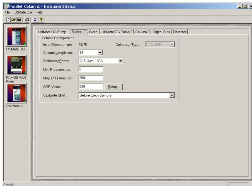
FIGURE 3-17 The Column 1 (Nano Column 1) Parameters Setup Window
