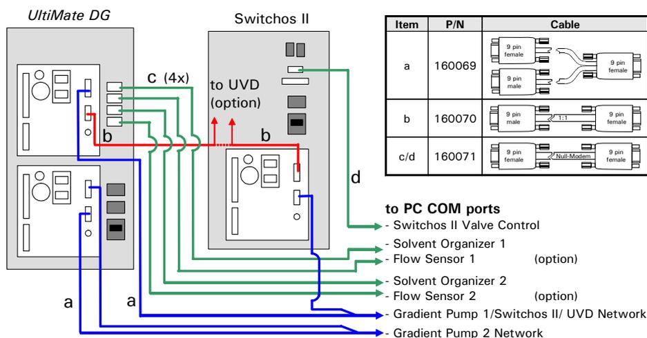
FIGURE 2-2 PC Connections of the UltiMate Dual Gradient System (with Flow Sensors) and Switchos
