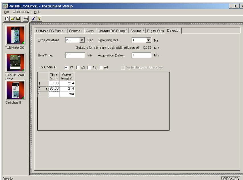
FIGURE 3-19 The UV Detector Setup Window
