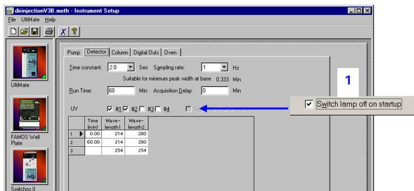
FIGURE 2-28 The UV Detector Setup Window
