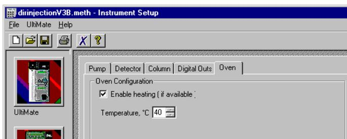
FIGURE 2-31 The Oven Setup Window
