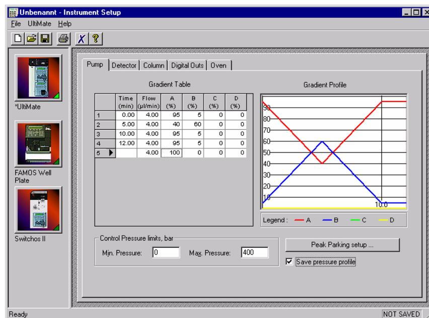
FIGURE 2-26 The Instrument Setup Window of the UltiMate System
