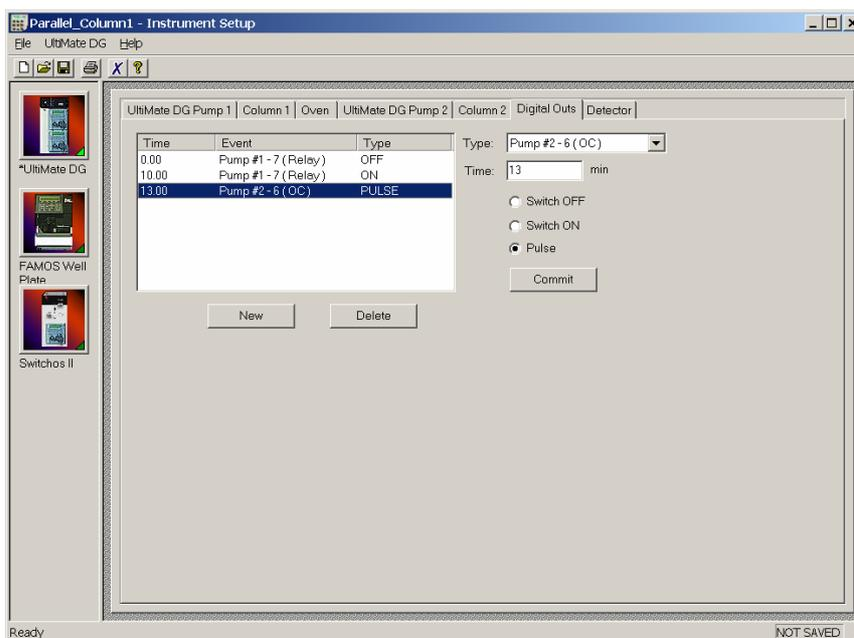
FIGURE 3-18 Controlling the Nano Switching Valve and the UV Autozero
