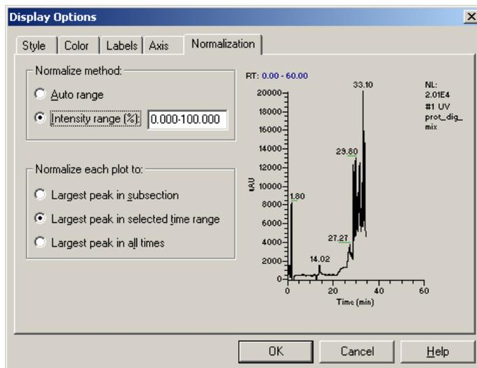
FIGURE 2-47 The Display Options Window (UV Data)
