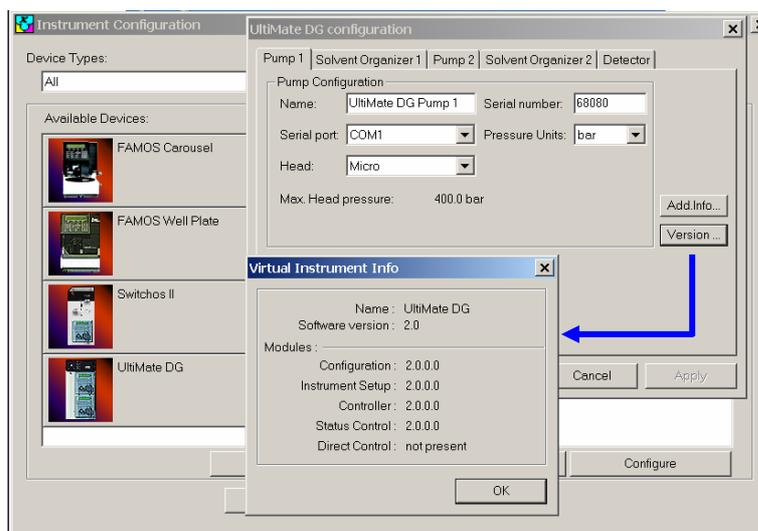
FIGURE 2-51 Reading the UltiMate Micropump Plug-In Version
