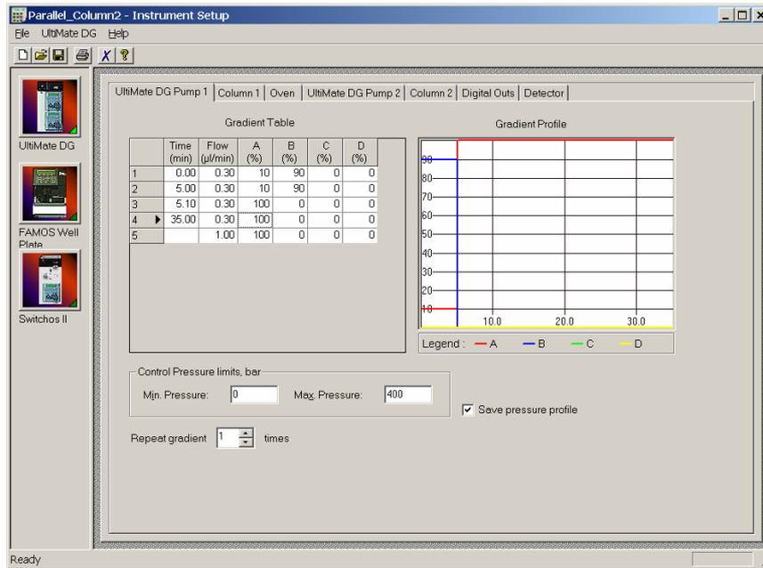
FIGURE 3-22 Gradient Program for the Gradient Pump 1 - Wash and Reconditioning
