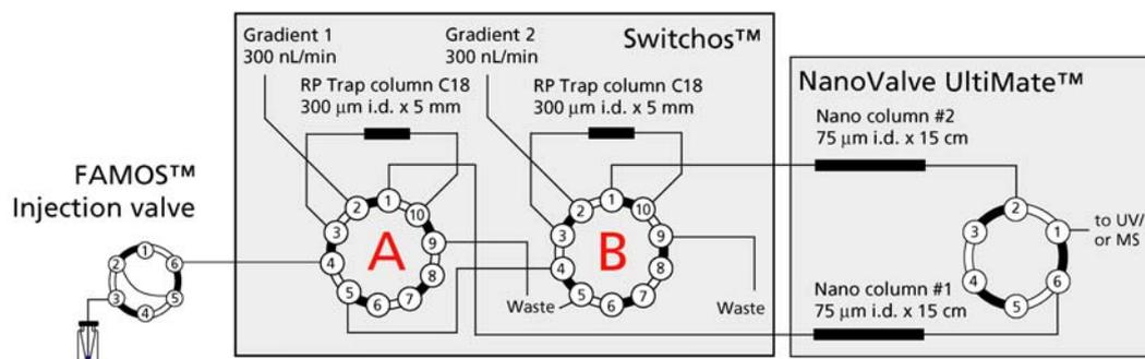
FIGURE 3-13 Fluidic Connections for the Parallel Nano-LC Application
