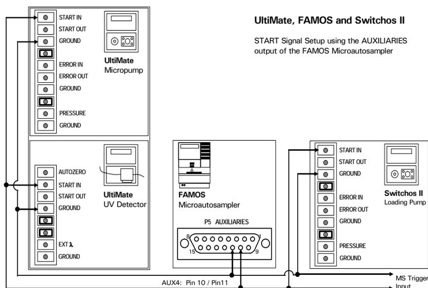
FIGURE 2-4 START Signal Setup – UltiMate, FAMOS and Switchos II
