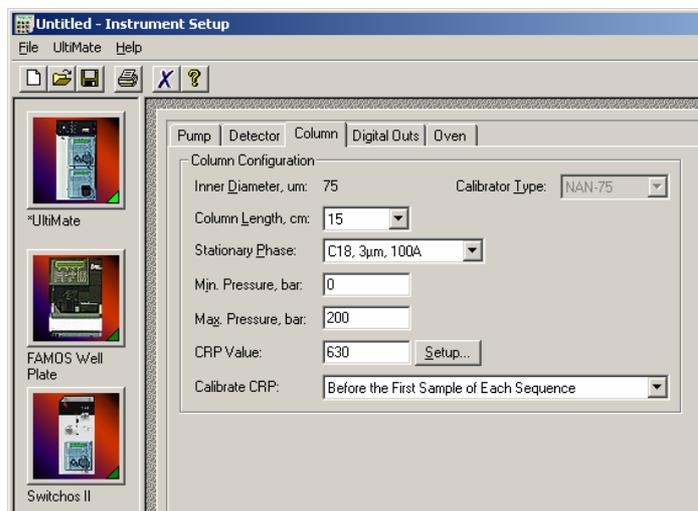
FIGURE 2-29 The Column Parameters Setup Window
