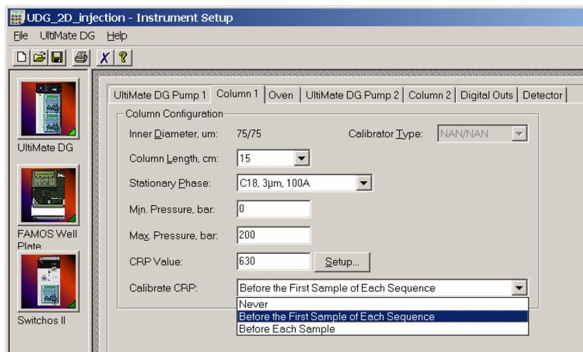
FIGURE 2-33 The Column 1 Parameters Setup Window
