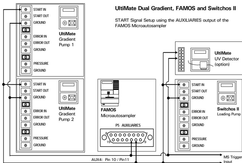
FIGURE 2-5 START Signal Setup – UltiMate Dual Gradient, FAMOS and Switchos II
