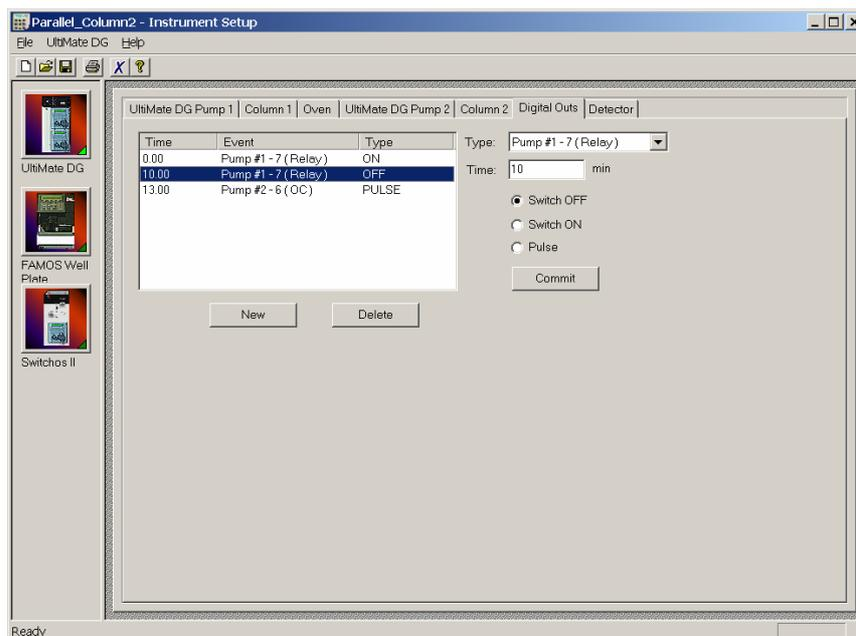
FIGURE 3-24 Controlling the Nano Switching Valve and the UV Autozero
