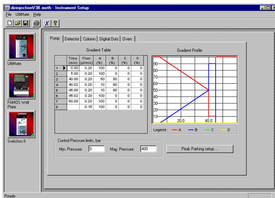
FIGURE 2-37 The Pump Setup Tab in the Instrument Setup Window
