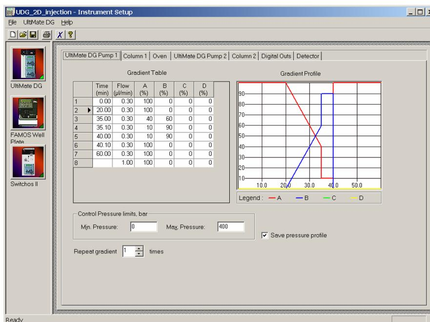
FIGURE 2-27 The Instrument Setup Window of the UltiMate Dual Gradient
