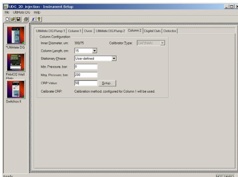
FIGURE 3-7 The Column 2 (IEX column) Parameters Setup Window
