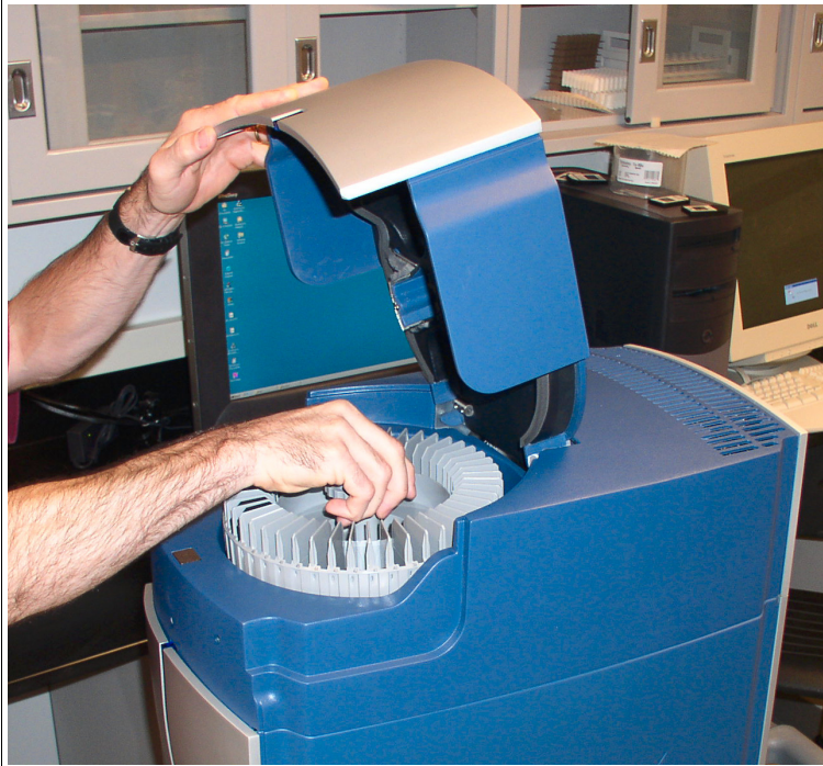
Figure 238 Inserting and turning the carousel. the carousel must be seated and flush with housing.
