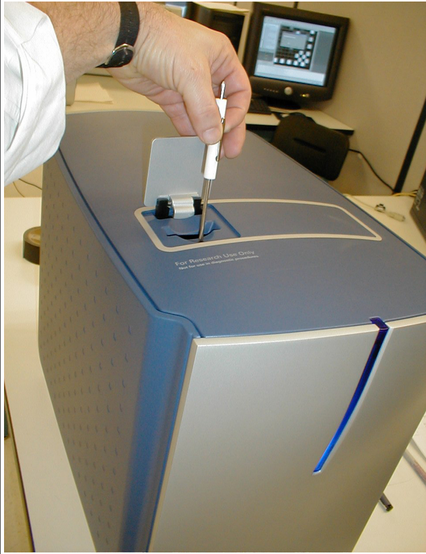
Figure 233 Turning the rescue screw
