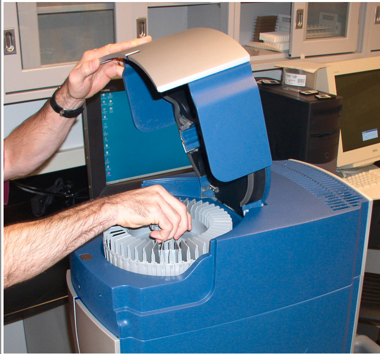
Figure 240 Inserting and turning the carousel. the carousel must be seated and flush with housing.
