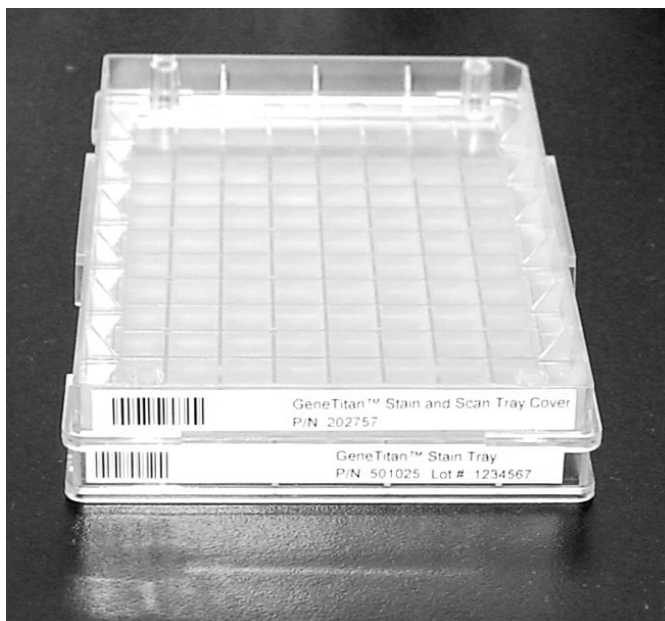
Figure 100 Stain Tray with Cover. Deionize the cover and the tray.
