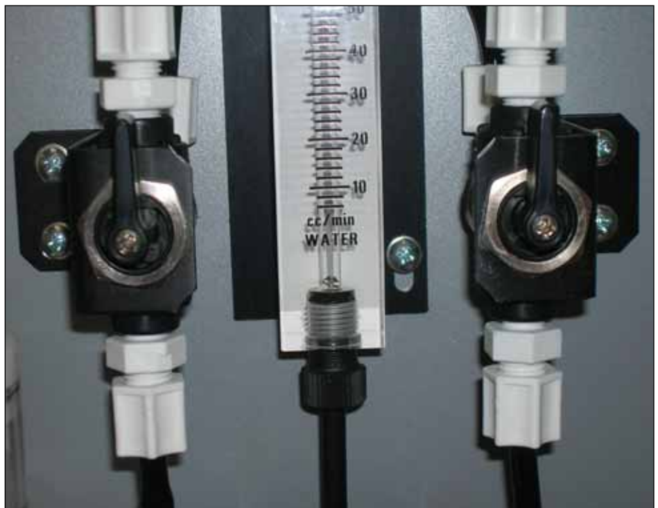
Figure IV-3 Calibration starting position showing both Left and Right air valves in the up position
