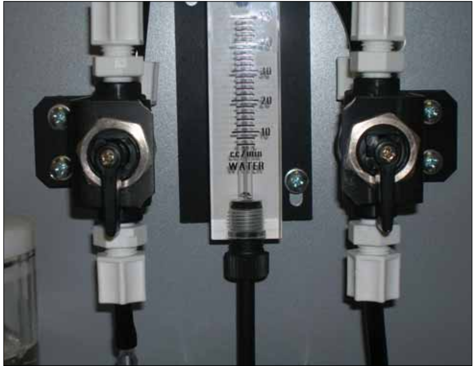
Figure IV-4 Measurement mode showing both Left and Right air valves in the down position
