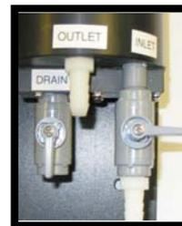
Drain Chamber, Shut off Inlet
