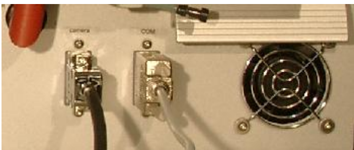
Fig. 7: plug in camera cable ('camera' adapter) and serial control cable ('COM' adapter).
