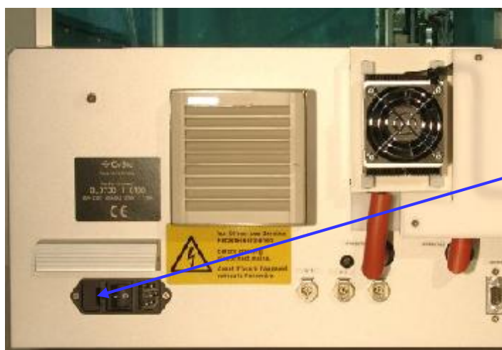
Fig. 21: Push back spring of fuse holder by applying a small screwdriver. Holder and fuse will then be automatically released and can be removed for replacing with new fuse.
