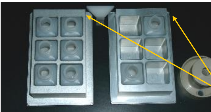
Fig. 10: Inserted reagent Reservoir Racks (here already containing reservoir bottles); ensure correct positioning marked by notched corners of the racks.
