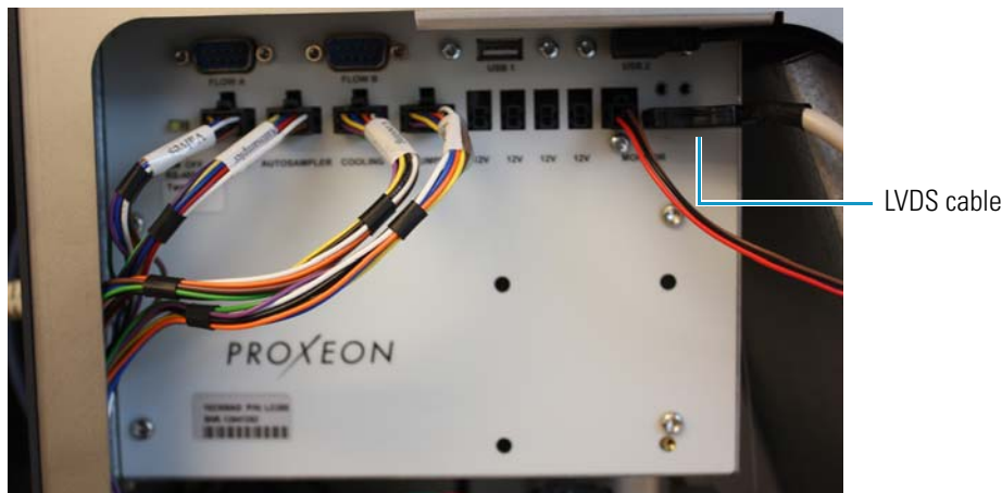
Figure 98. Cables connected to the computer box in the EASY-nLC II instrument
