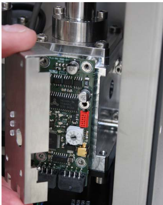
Figure 177. Removing the PCB shield (PLU model pump)
