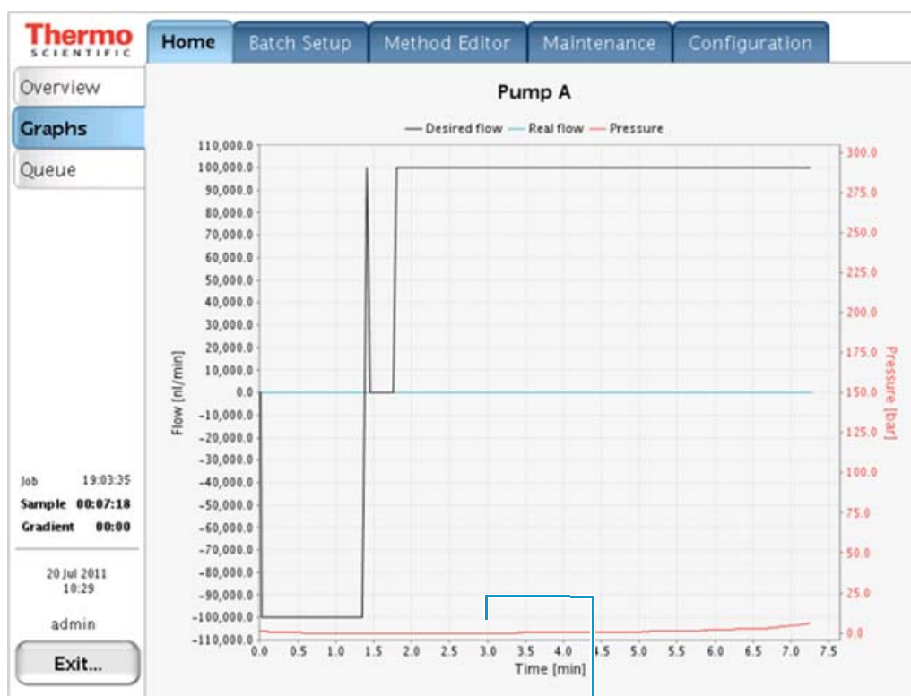
Figure 193. Leak test profile for pump A
