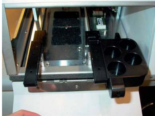
Figure 156. Aligning the arms of the autosampler bed
