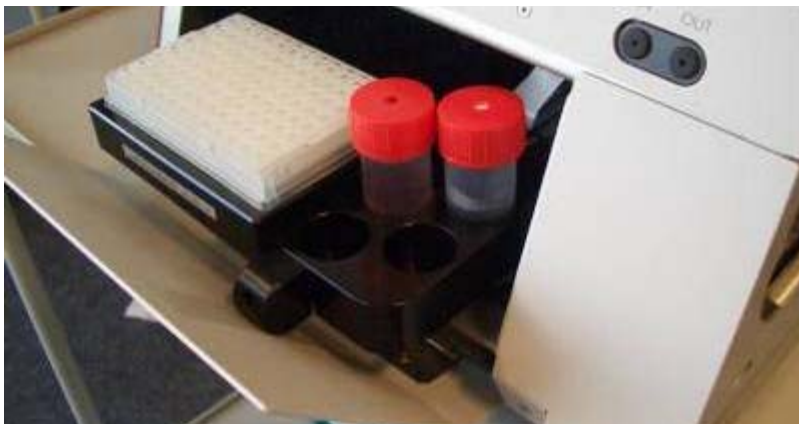
Figure 5. Tray compartment for the ASA autosampler model (viewed from above)
