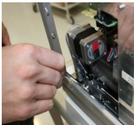
Figure 119. Removing the screw from the right side of the autosampler
