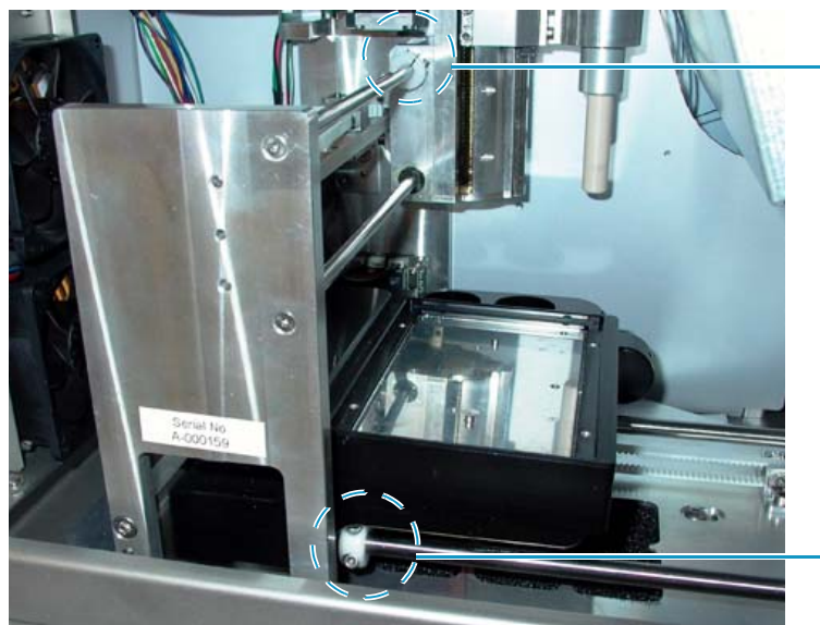
Figure 258. (ASA autosampler only) Transport collar location
