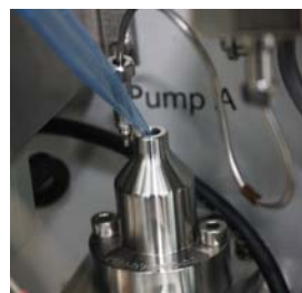
Figure 7. Adding solvent to the pump head
