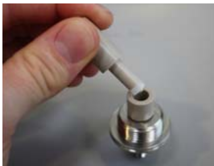
Figure 55. Inserting the piston seal tool into the guide (PLF model pump)
