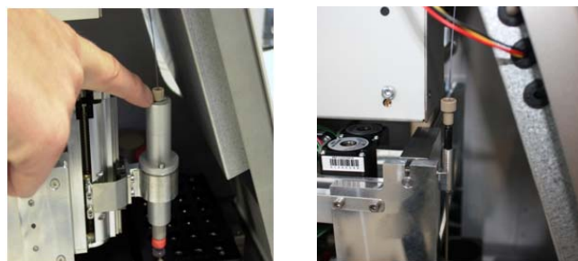
Figure 7. Autosampler needle connected to the z -axis needle holder
