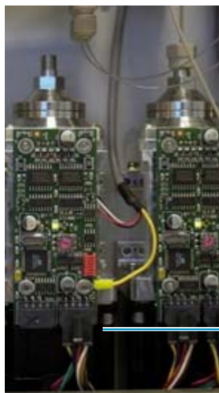
Figure 108. P-Bus communication cables connected to the pump PCB of the PLF pump
