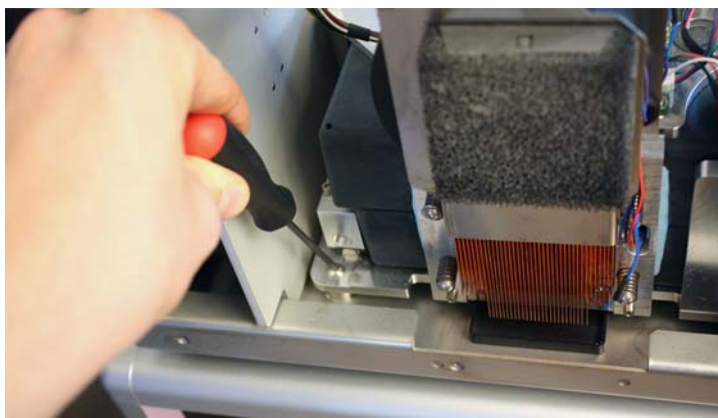
Figure 120. Removing the screw from the back left of the autosampler
