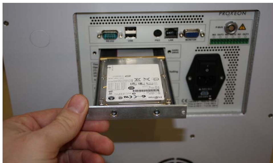
Figure 93. Pulling out the hard-drive drawer
