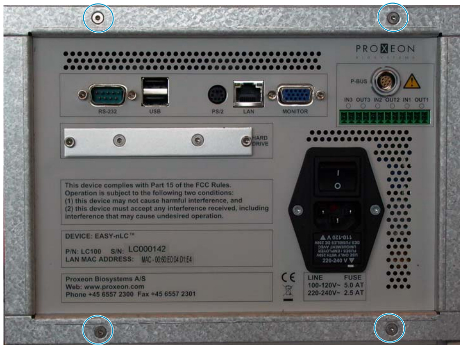
Figure 101. Screws to remove from the computer box
