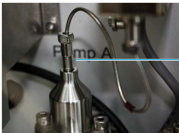
Figure 162. Fitting on the pump head
