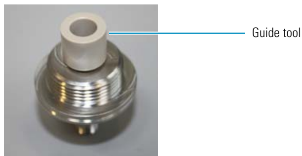
Figure 53. Guide tool inserted into the pump head flange (PLF model pump)
