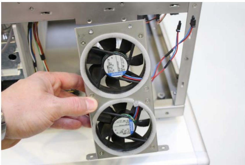
Figure 124. Removing the fan assembly and cables
