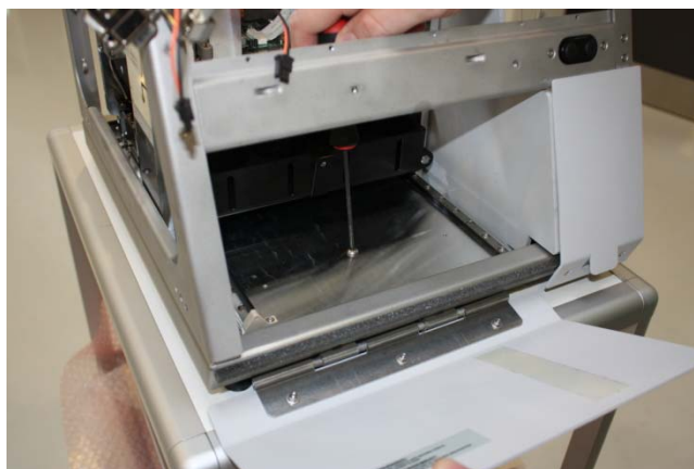
Figure 135. Securing the front screw
