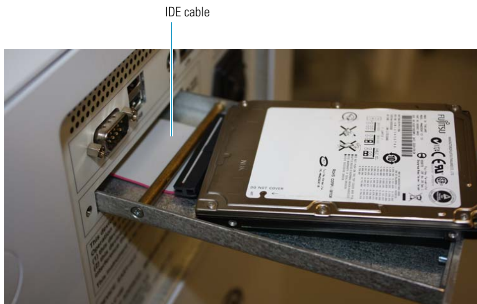
Figure 95. Hard drive unplugged from the IDE cable
