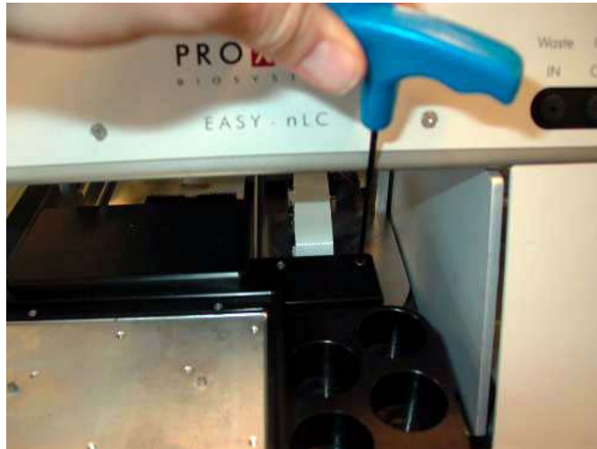
Figure 150. Removing the lid
