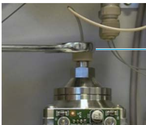
Figure 165. Externally threaded pump head for a PLF model pump
