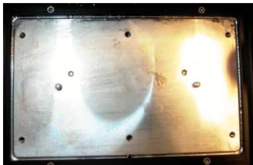
Figure 241. Tray for the ASA model autosampler
