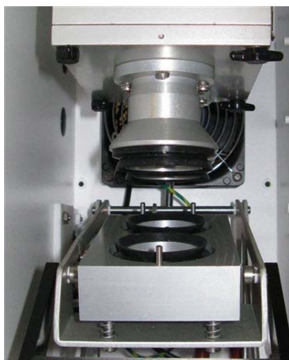
Figure 10–13. Upper and Lower V-Seals on Partisol 2000 i -D
