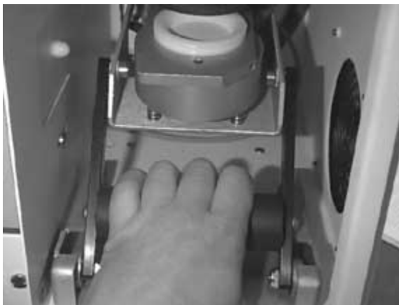
Figure 10–10. Pulling Backward on the Handle of the Filter Exchange Mechanism
