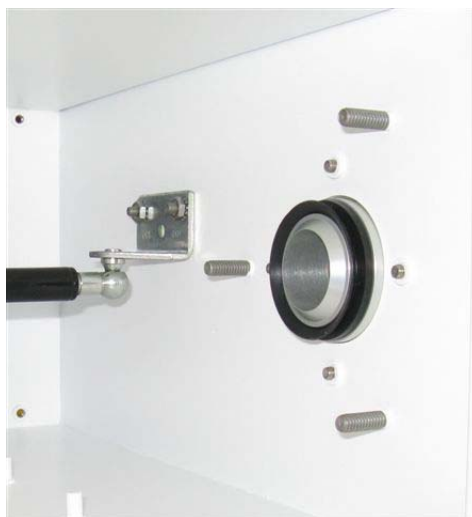
Figure 10–14. V-Seal on Inlet Adapter Tube on 2000 i -D
