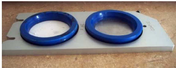
Figure 8–9. Solid Leak Check Cassette in the Front Position
