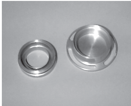
Figure 10–5. Upper and Lower Sections of the Impactor Assembly (on left and right sides of figure)
