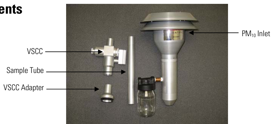
Figure 4–1. PM 2.5 VSCC Cyclone, VSCC Adapter, Sample Tube, and U.S. EPA PM 10 Inlet
