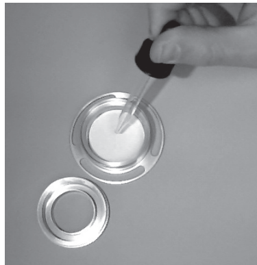
Figure 10–6. Coating the 37 mm Glass Filter with Oil
