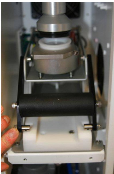
Figure 10–11. Lifting the Rollers through the Guide Slots
