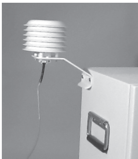
Figure 2-4. Ambient Temperature Probe Assembly Mounted on the Enclosure
