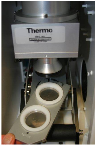
Figure 3–8. Inserting/Removing Filter Cassette in Filter Cassette Carrier in the Partisol 2000i-D
