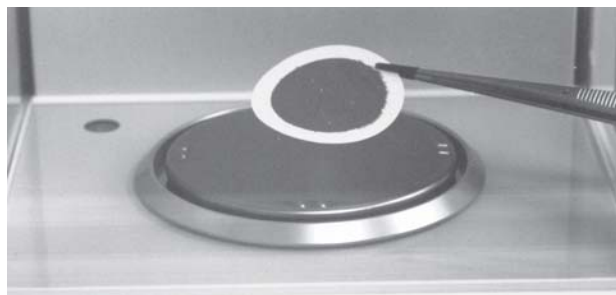
Figure 3–10. Placing a Used 47 mm Filter on a Balance
