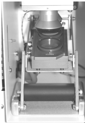
Figure 7-4. Filter Cassettes and Carrier Installed into Filter Exchange Mechanism in the Partisol 2000i-D
