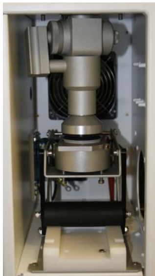
Figure 4–13. Partisol 2000i PM 2.5 with VSCC
