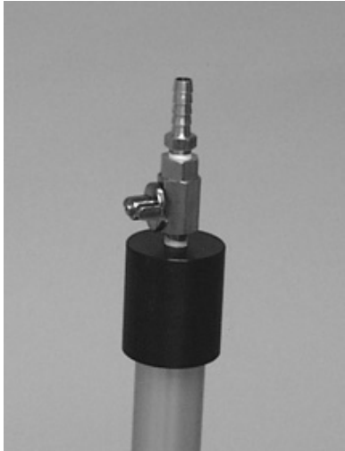
Figure 7-5. Flow Audit Adapter Installed
