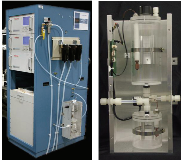
Figure 1–9. Hydrator System Mount and Close-up View
