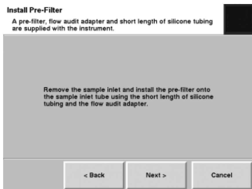
Figure 5-82. Install Pre-Filter screen.
