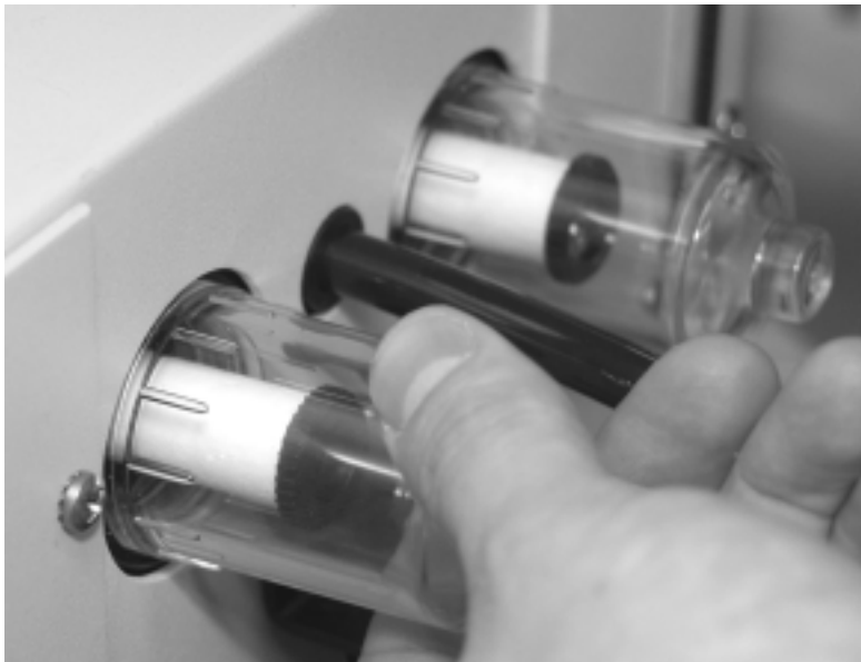
Figure 5-30. Removing the fine and coarse filter covers.
