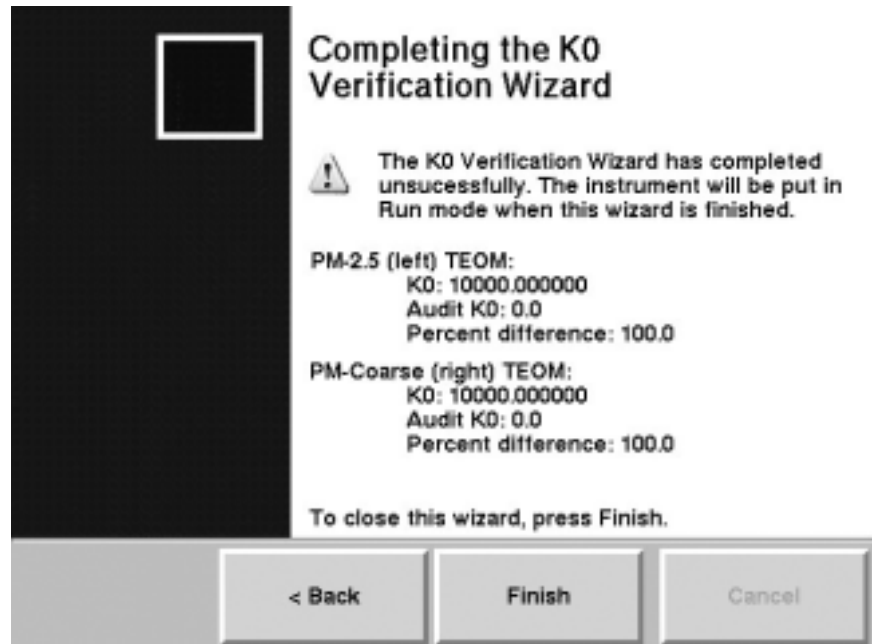
Figure 5-90. Completing the K0 Verification Wizard screen with a fail message.
