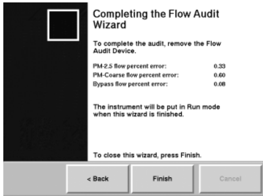
Figure 5-61. Finish screen with flow audit results.
