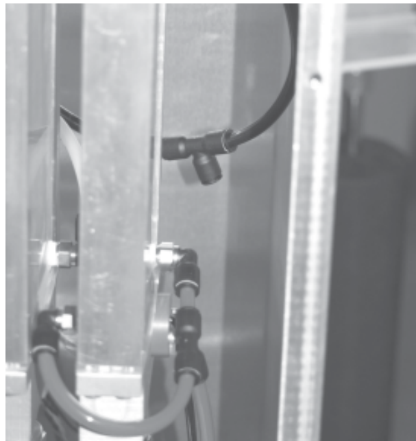
Figure 5-40. Main dryer vacuum line removed from T-fitting.
