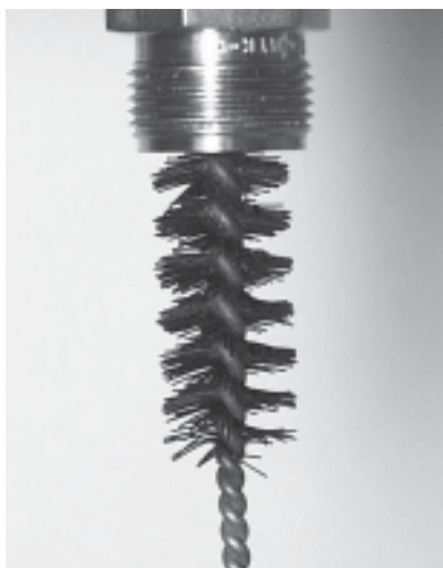
Figure 5-47. Cleaning the valve with the valve brush.
