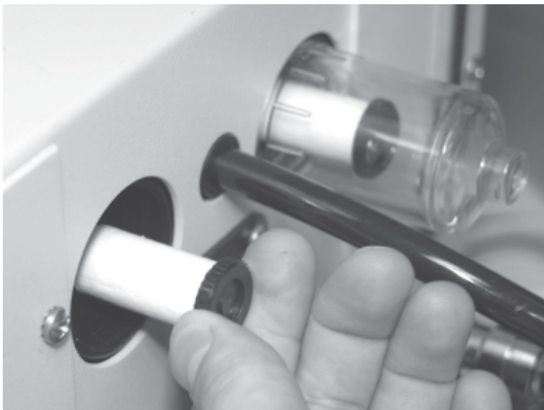
Figure 5-31. Removing the filter mounts.
