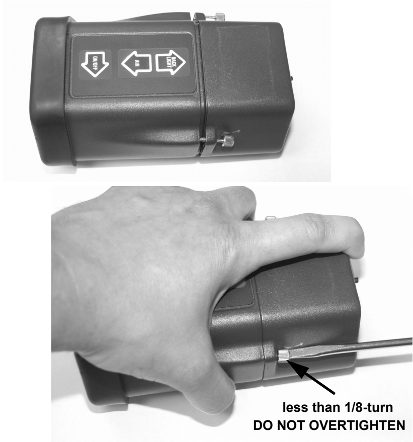
Figure 2-3 Connecting the Housings
