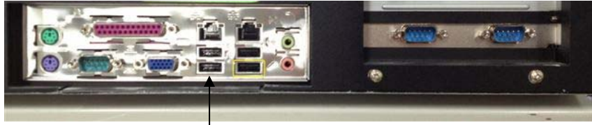
Temperature Controller Connection
