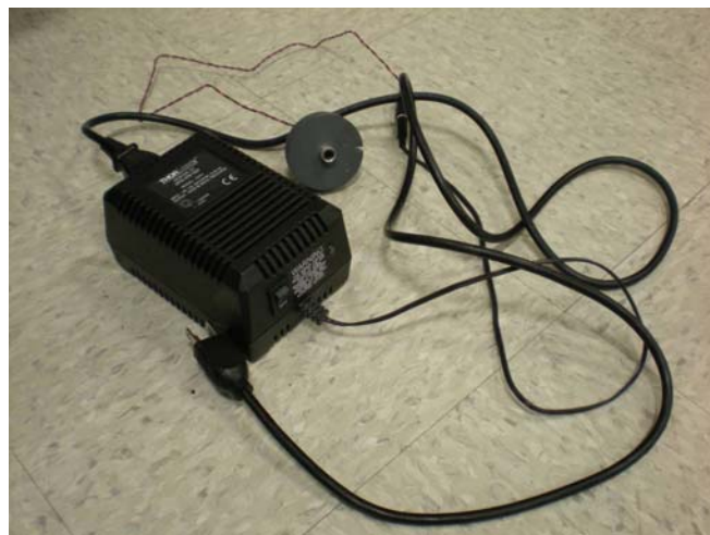
Figure 5–35. Visible Laser Module for Gas Cell Alignment
