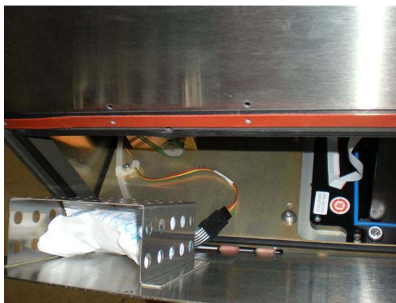
Figure 5-4. Replacing the Desiccant
