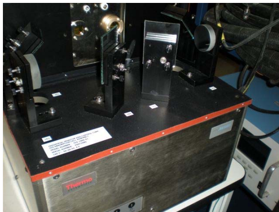
Figure 5–15. Corner Screws on Coupling Optics Plate
