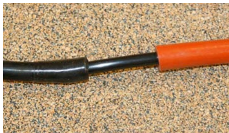
Figure 5–20. Installing the flow/audit/tubing adapter
