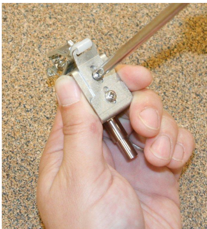
Figure 5–13. Loosen screws on rear of bracket
