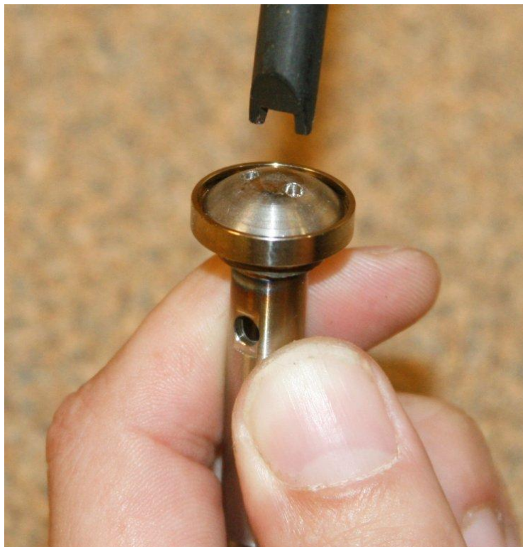
Figure 5–16. Remove sealing screw using inlet spanner tool
