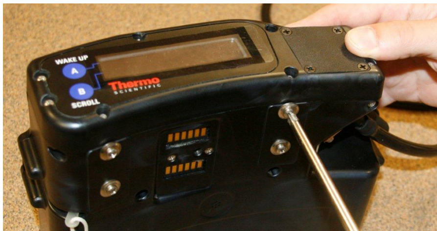
Figure 2–2. Remove sealing screws. Retain for future use.
