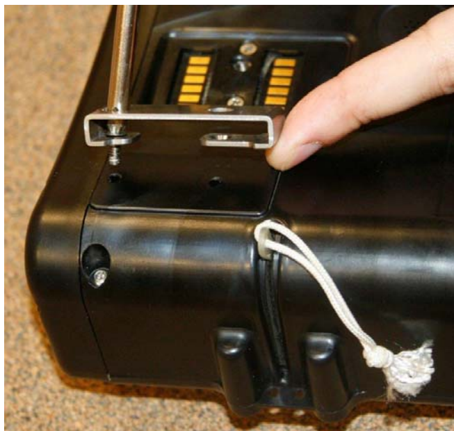
Figure 2–3. Installing belt loops on side of instrument. Note that small tab is at the top of the belt loop.
