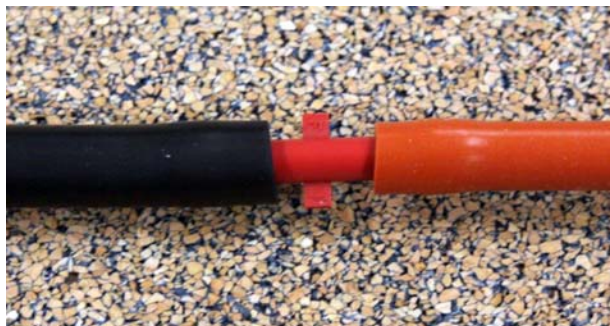
Figure 5–54. Red orifice installed
