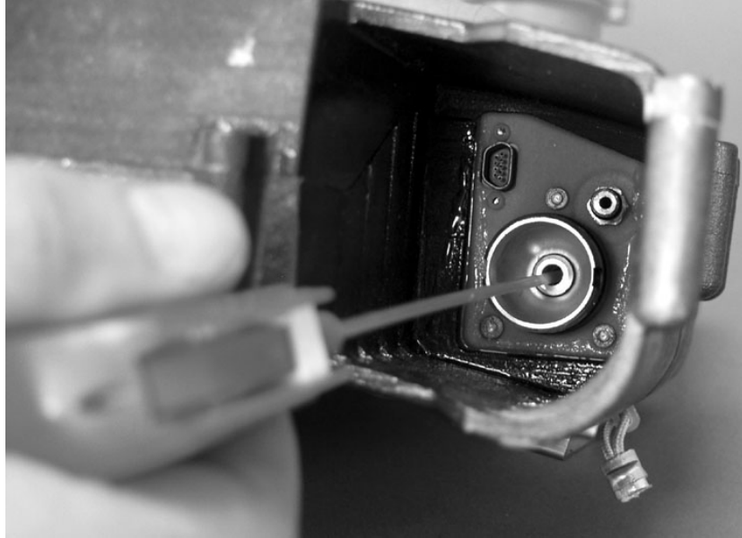
Figure 5-10. Clean the bell-shaped inlet with air
