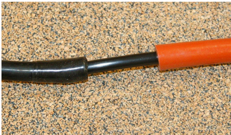
Figure 5-49. Install tubing adapter into the sample line
