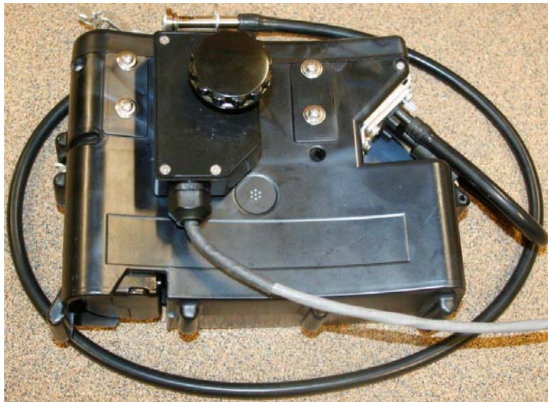
Figure 2–7. Locking in the PDM3700 charger connection
