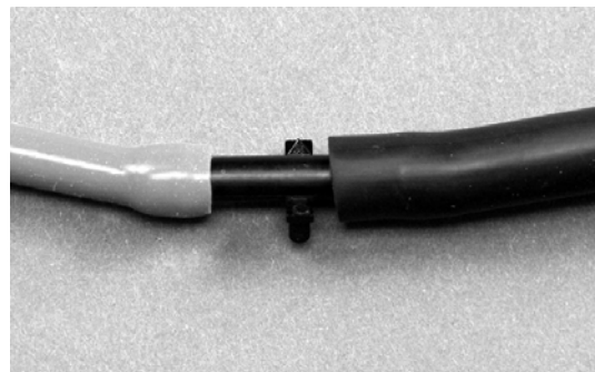
Figure 5–53. Black orifice installed in sample line and flow meter tubing
