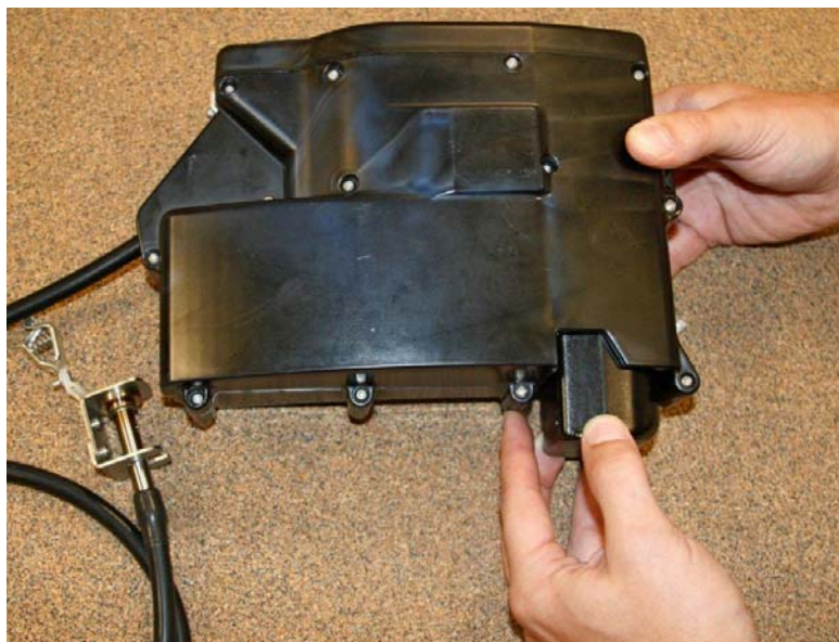
Figure 2–10. Removing the mass transducer
