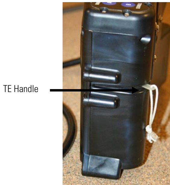
Figure 2–9. Slide the PDM3700 handle to the right
