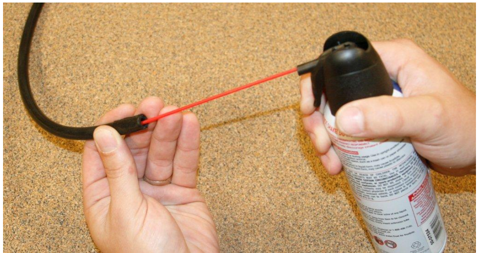
Figure 5-11. Direct a stream of air through the sample line
