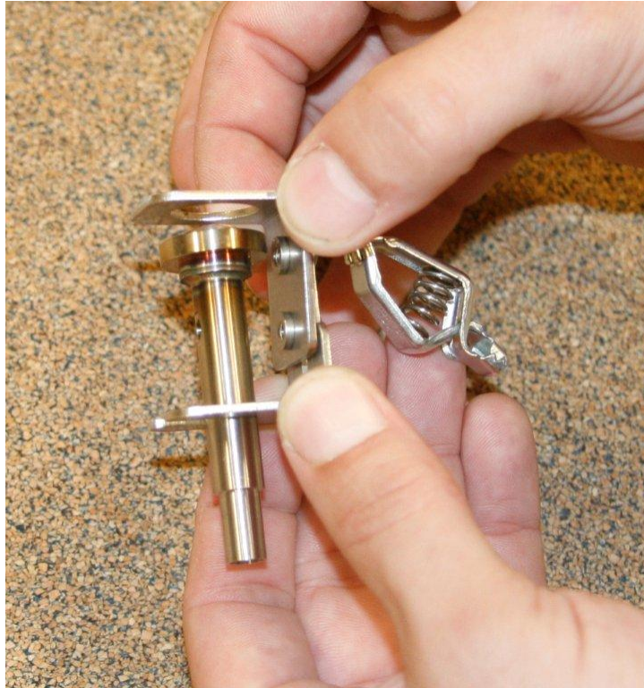
Figure 5–14. Open sample inlet assembly bracket
