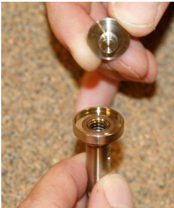
Figure 5–18. Inspect o-ring in top of inlet for damage
