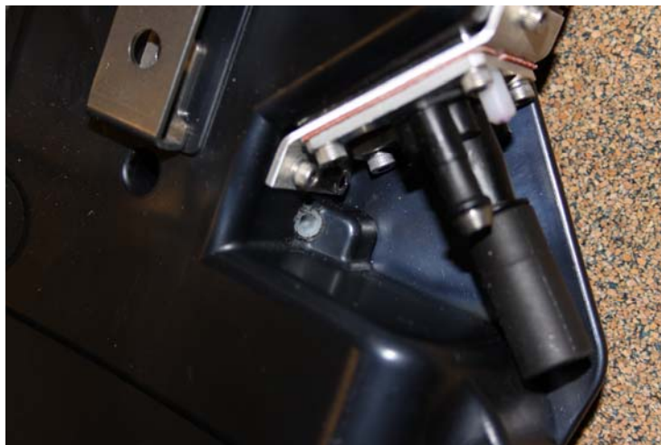
Figure 5–37. Pump exhaust muffler
