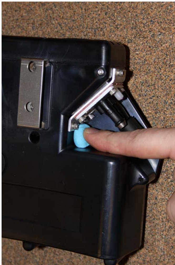
Figure 5–38. Placing the leak check putty
