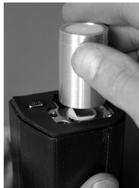
Figure 2–12. Removing the TEOM filter with the filter tool
