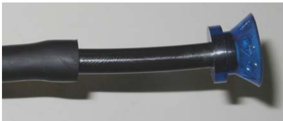
Figure 5–39. Leak check suction cup installed in sample line
