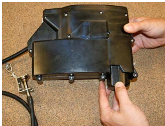
Figure 5-2. Removing the mass transducer
