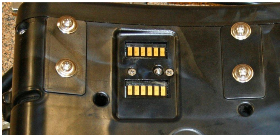
Figure 2-5. Charger connection on the back of the PDM3700 unit
