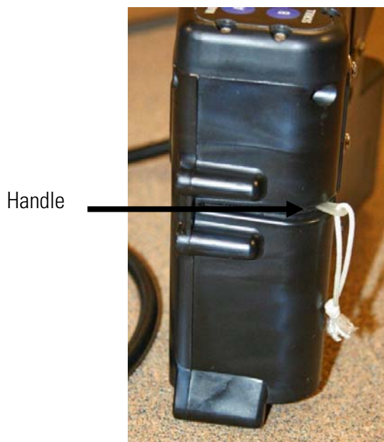
Figure 5-1. Sliding the handle right to release the mass transducer
