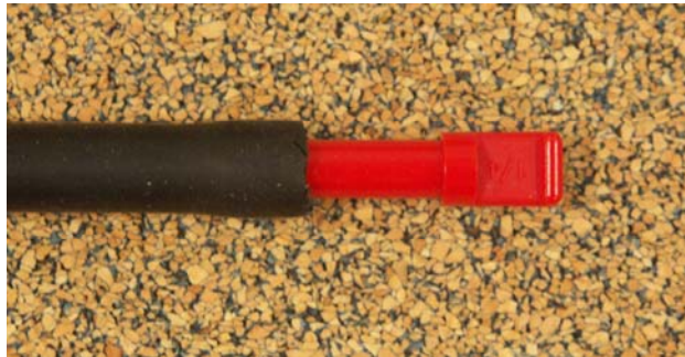
Figure 5–36. Insert sample line plug into tubing
