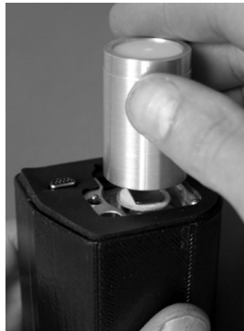
Figure 5–4. Removing the TEOM Filter with the Filter Tool
