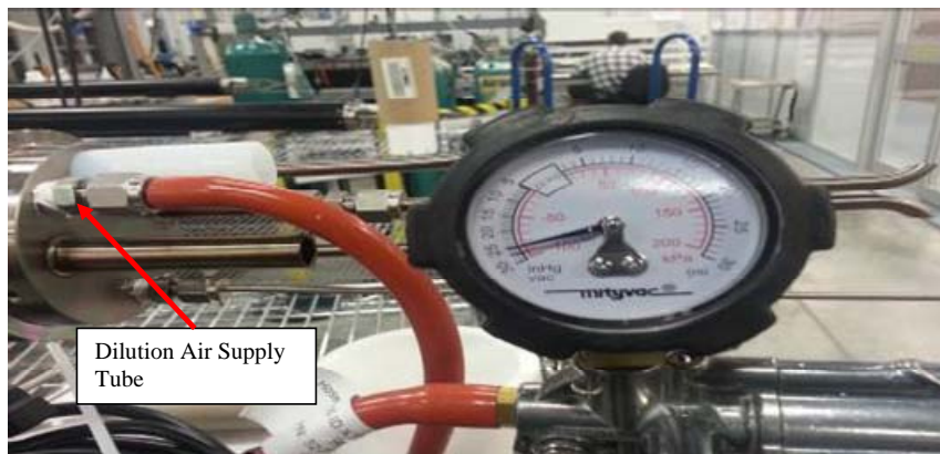
Figure 5-37. Isolated Dilution Assembly of the Mantle
