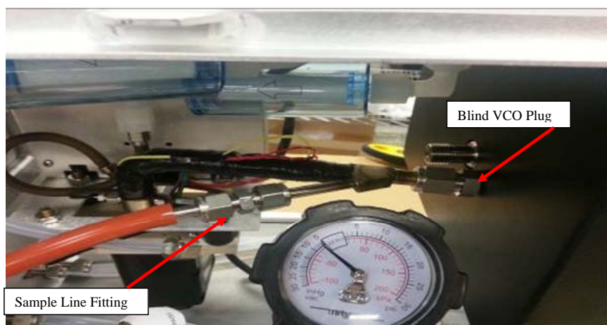
Figure 5–29. Sample Line Connection with Capped Air Tube – Blind VCO Plug
