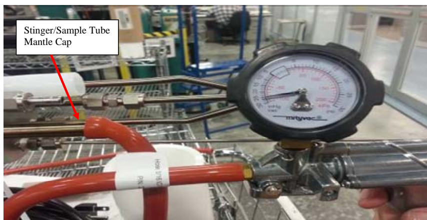
Figure 5-38. Isolated Stinger/Sample Assembly of the Mantle
